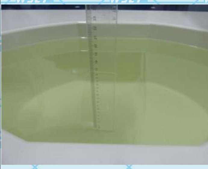
Photo 14: 1800~1900MHz Liquid Depth \geq 15.0\text{cm}
