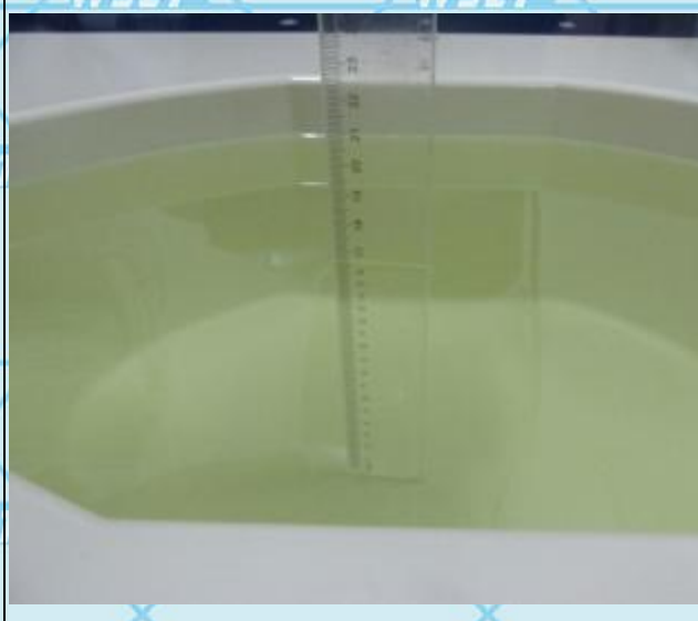
Photo 15: 2450MHz Liquid Depth \geq 15.0\text{cm}
