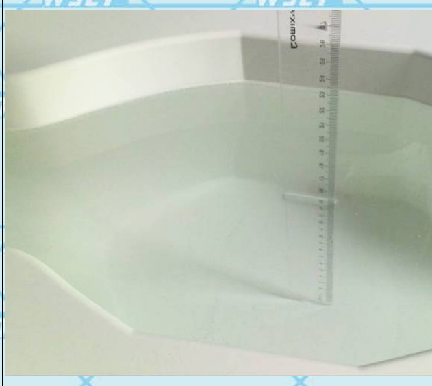
Photo 15: 2450MHz Liquid Depth \geq 15.0\text{cm}
