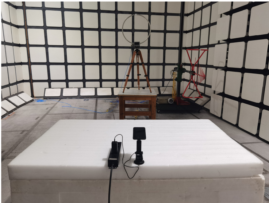
Radiated Emissions Side View (Below 30MHz)
