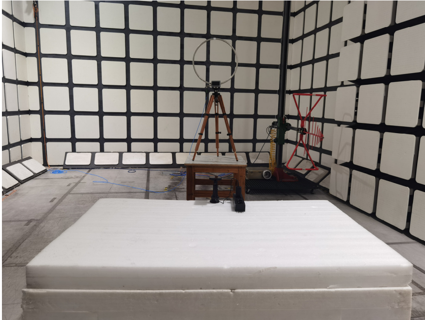
Radiated Emissions Front View (Below 30MHz)
