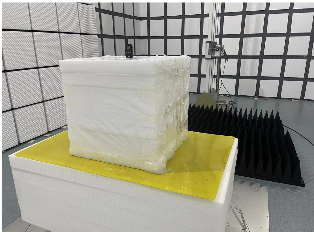
Photo of Radiated Emission Measurement (Above 1G)
