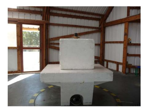
Photograph No.6 Setup for 20 dB OBW and band edge emission measurements
