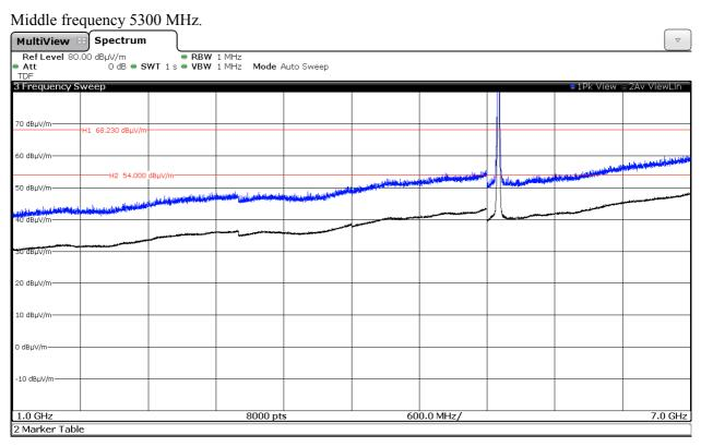
Note: The peak above the limit is the carrier frequency. This plot is valid for Chain A, Chain B, Chain A+B.
