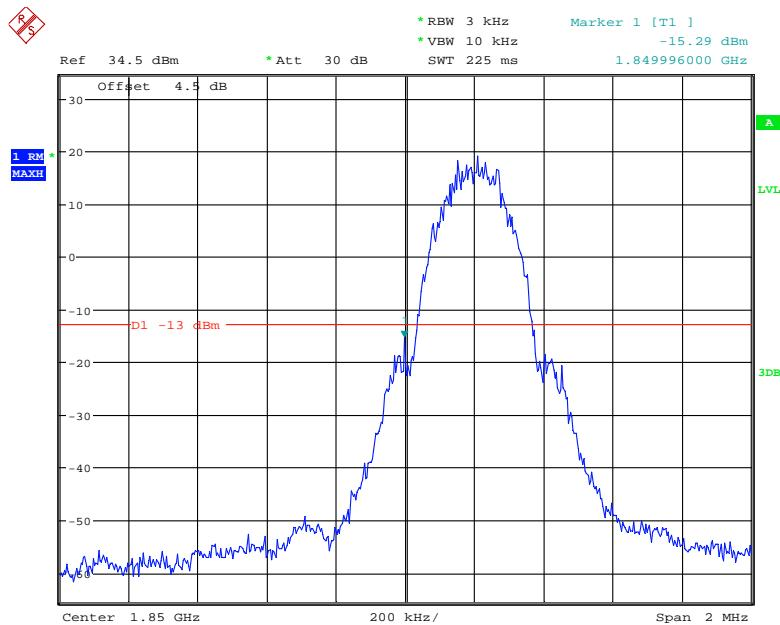
**GSM 1900, Right Band Edge**
