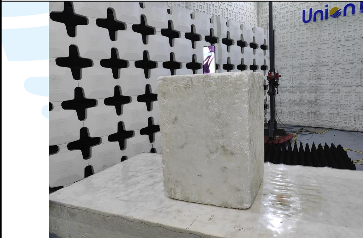
Radiated emission Test Setup (Above 1 GHz)
