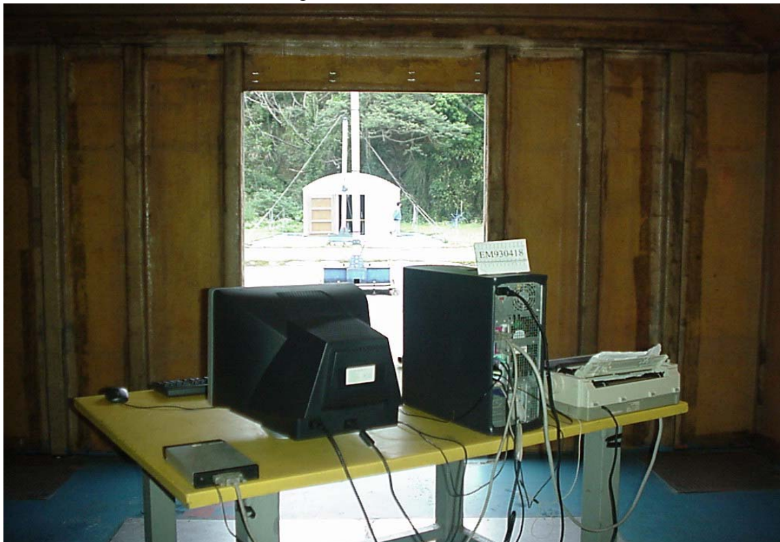
SETUP WITH MAXIMUM DETECTED EMISSION AT HORIZONTAL POLARIZATION
