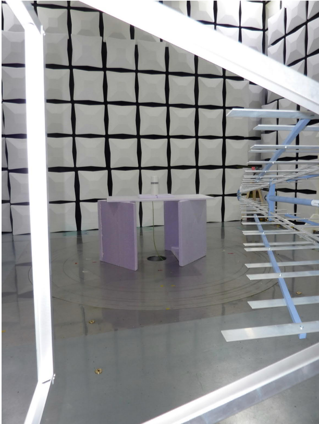
Test setup semi anechoic chamber TX spurious emissions from 30 MHz to 1 GHz
