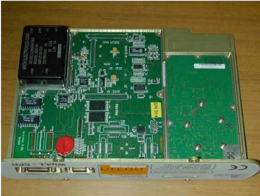
FCC ID:PIDMARCONI; SPR-2.4 inside view without covers
