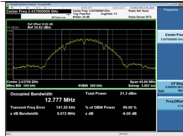
6 dB Bandwidth plot (802.11n_HT20-CH 6)
