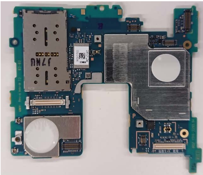
Internal PWB with Shield cases (Front-side)
