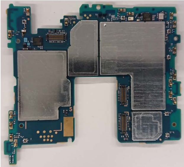
Internal PWB with Shield cases (Rear-side)
