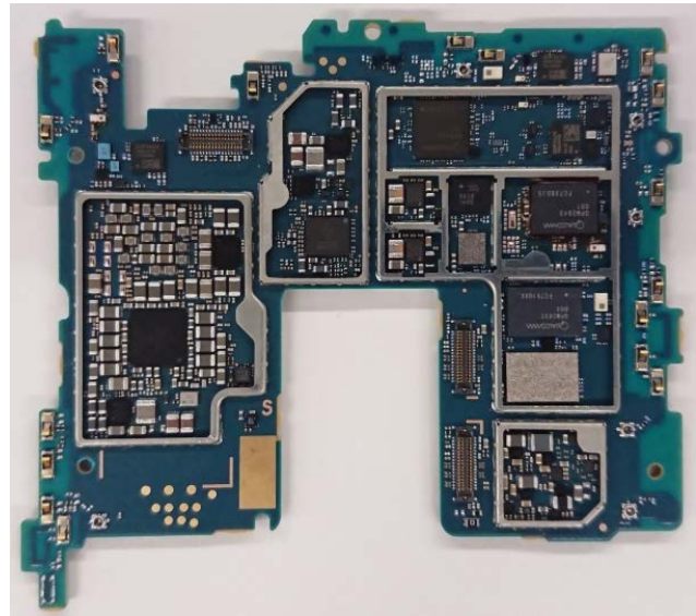
Internal PWB without Shield cases (Rear-side)
