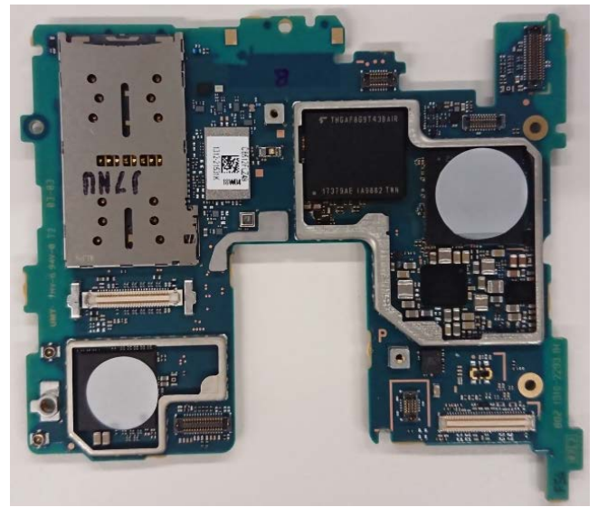
Internal PWB without Shield cases (Front-side)
