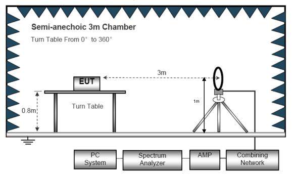
(B) Radiated Emission Test-Up Frequency 30MHz~1GHz
