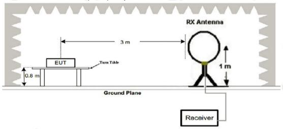
2. Radiated Emission Test-Up Frequency 30MHz~1GHz
