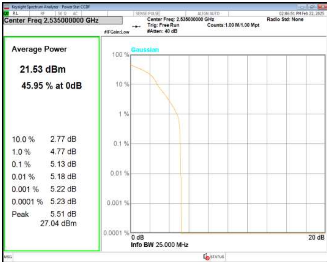
Band7 QPSK BW=5MHz Channel=21425 RB Size=1 Position=#0
