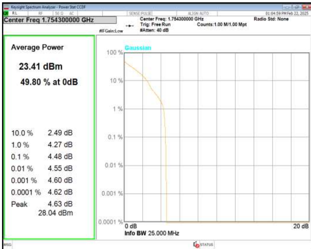
Band4 16QAM BW=1.4MHz Channel=20393 RB Size=1 Position=#0
