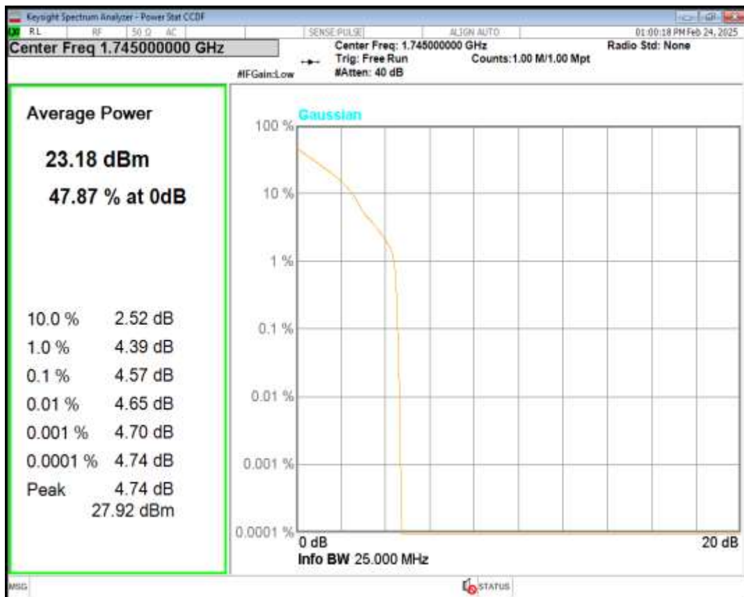
Band66 16QAM BW=10MHz Channel=132322 RB Size=1 Position=#0
