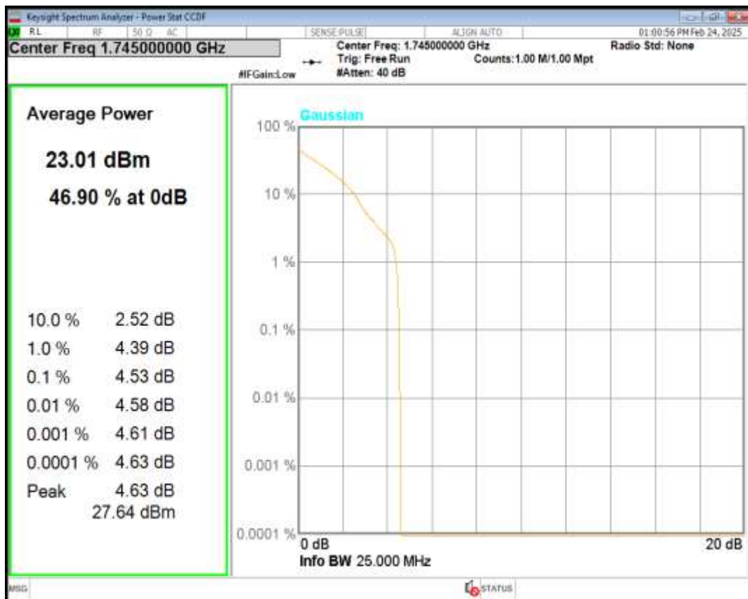
Band66 16QAM BW=20MHz Channel=132322 RB Size=1 Position=#0
