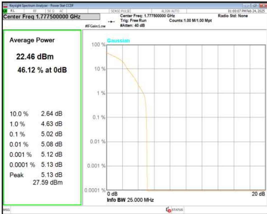
Band66 QPSK BW=10MHz Channel=132022 RB Size=1 Position=#0
