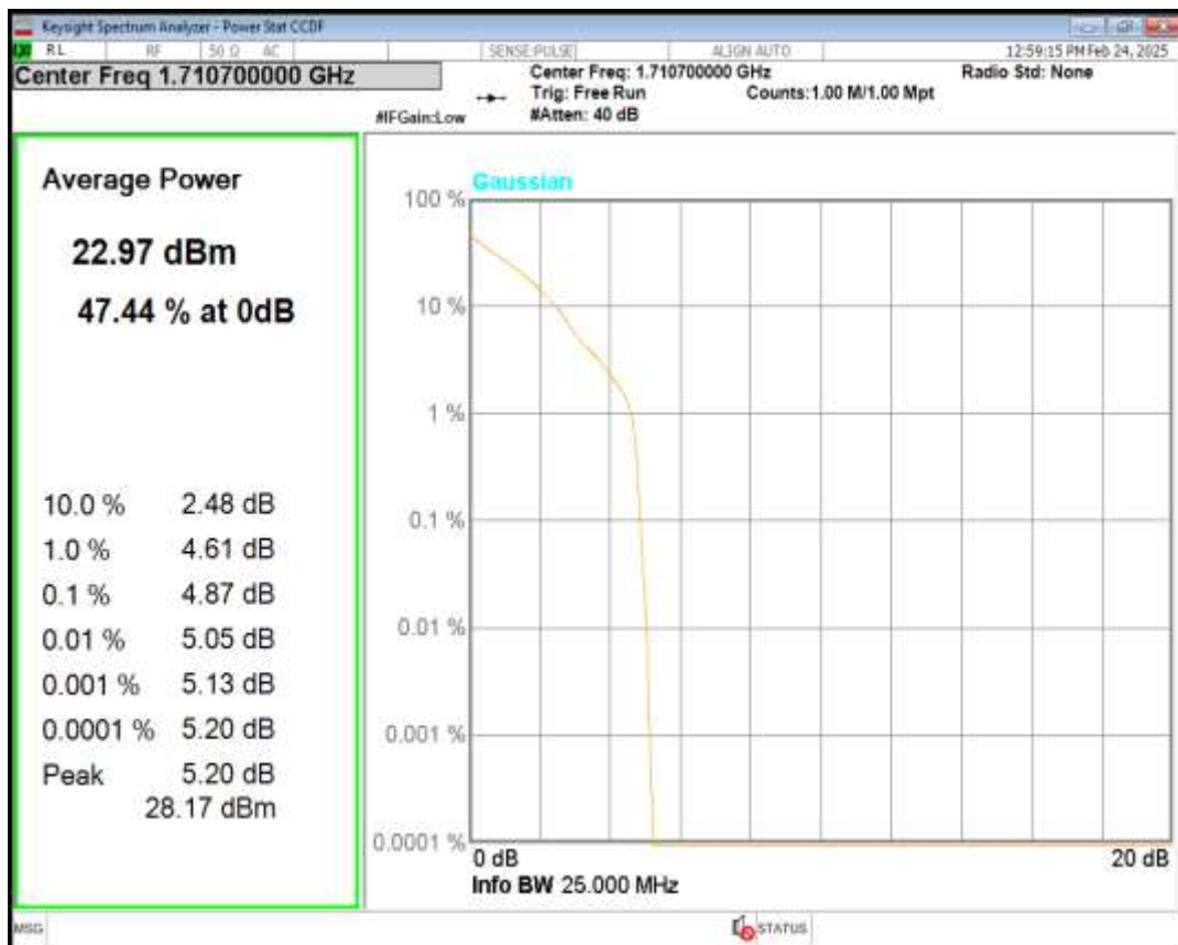
Band66 16QAM BW=1.4MHz Channel=131979 RB Size=1 Position=#0
