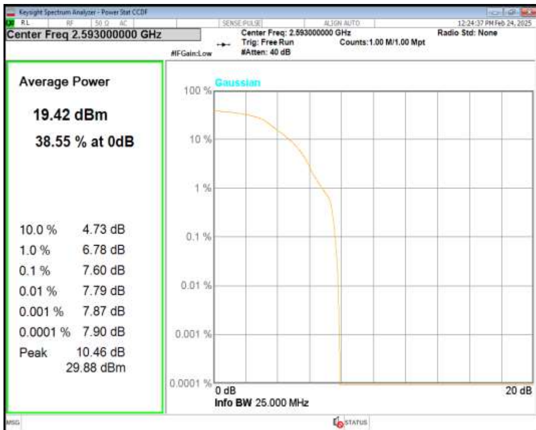
Band41 16QAM BW=20MHz Channel=40620 RB Size=1 Position=#0
