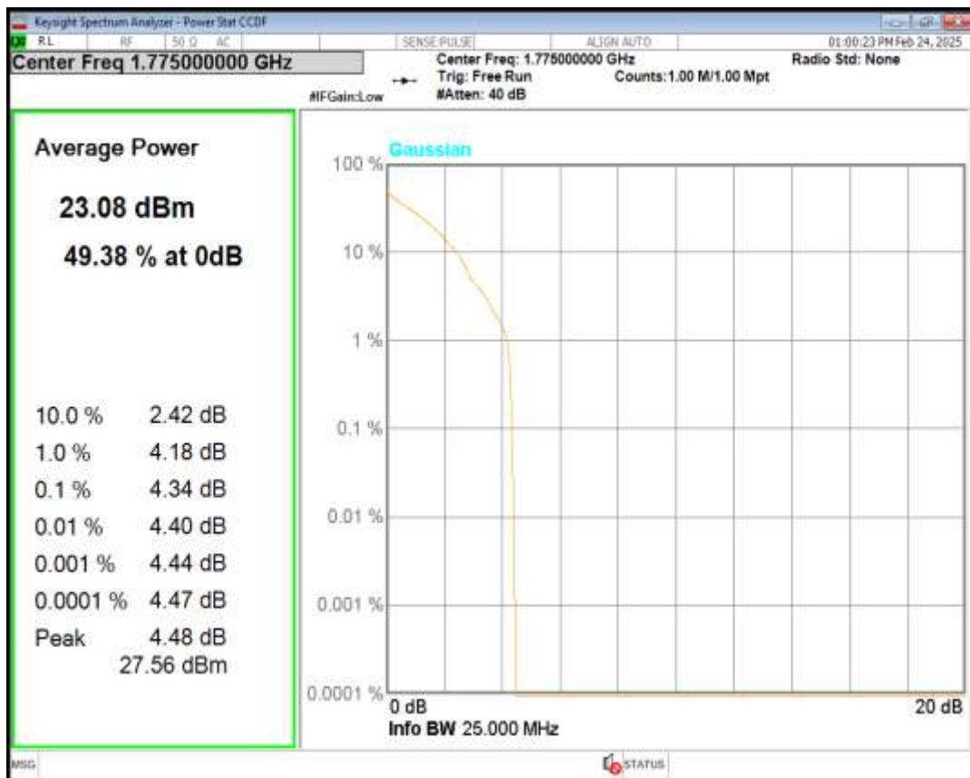
Band66 16QAM BW=10MHz Channel=132622 RB Size=1 Position=#0
