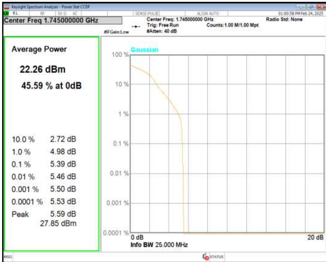
Band66 QPSK BW=20MHz Channel=132572 RB Size=1 Position=#0
