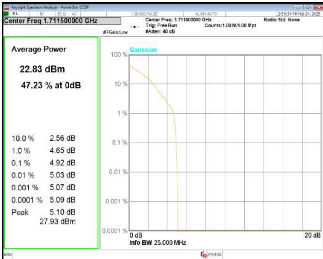
Band66 16QAM BW=3MHz Channel=131987 RB Size=1 Position=#0
