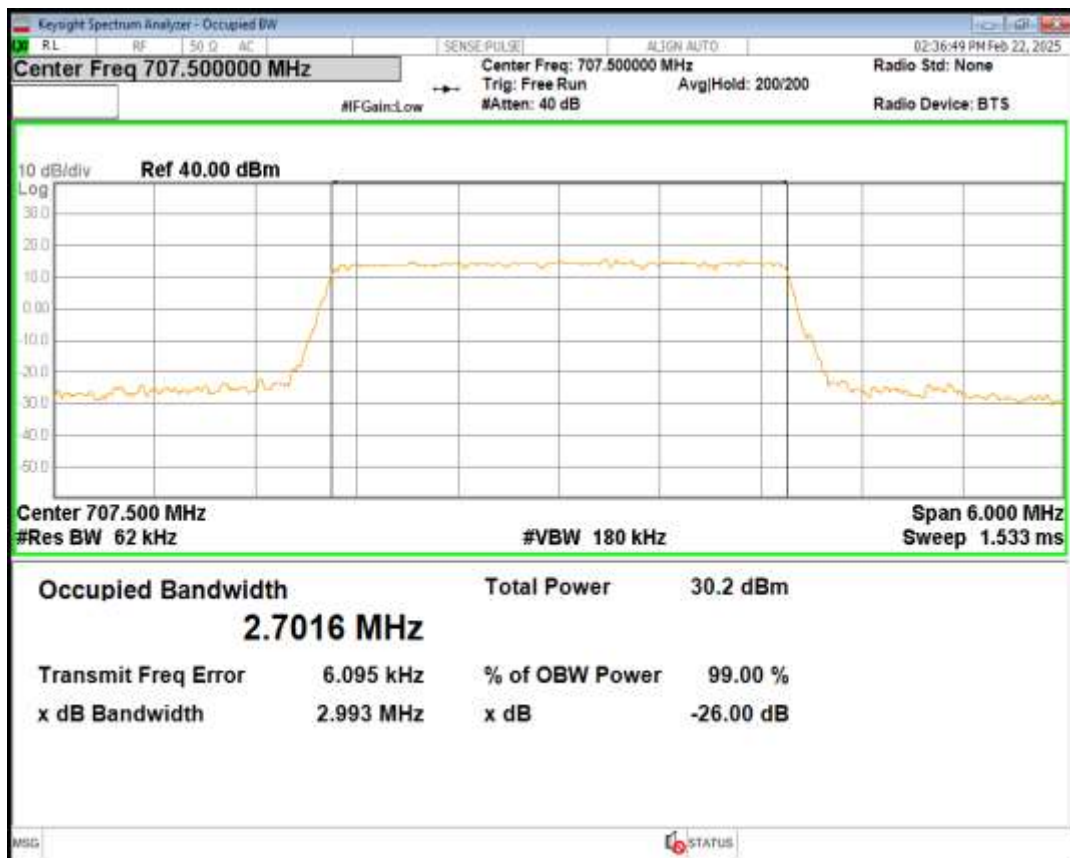
Band12 QPSK BW=3MHz Channel=23165 RB Size=15 Position=#0
