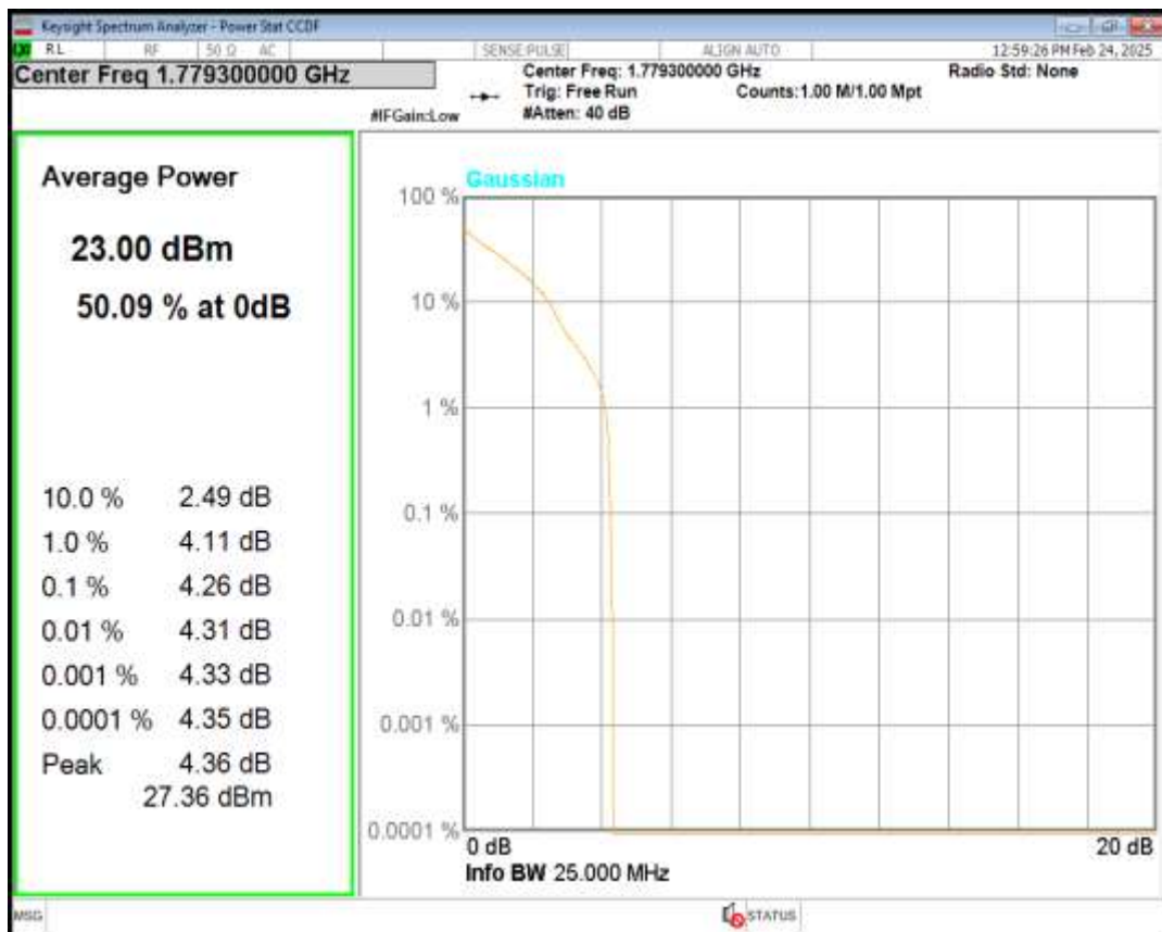
Band66 16QAM BW=1.4MHz Channel=132665 RB Size=1 Position=#0
