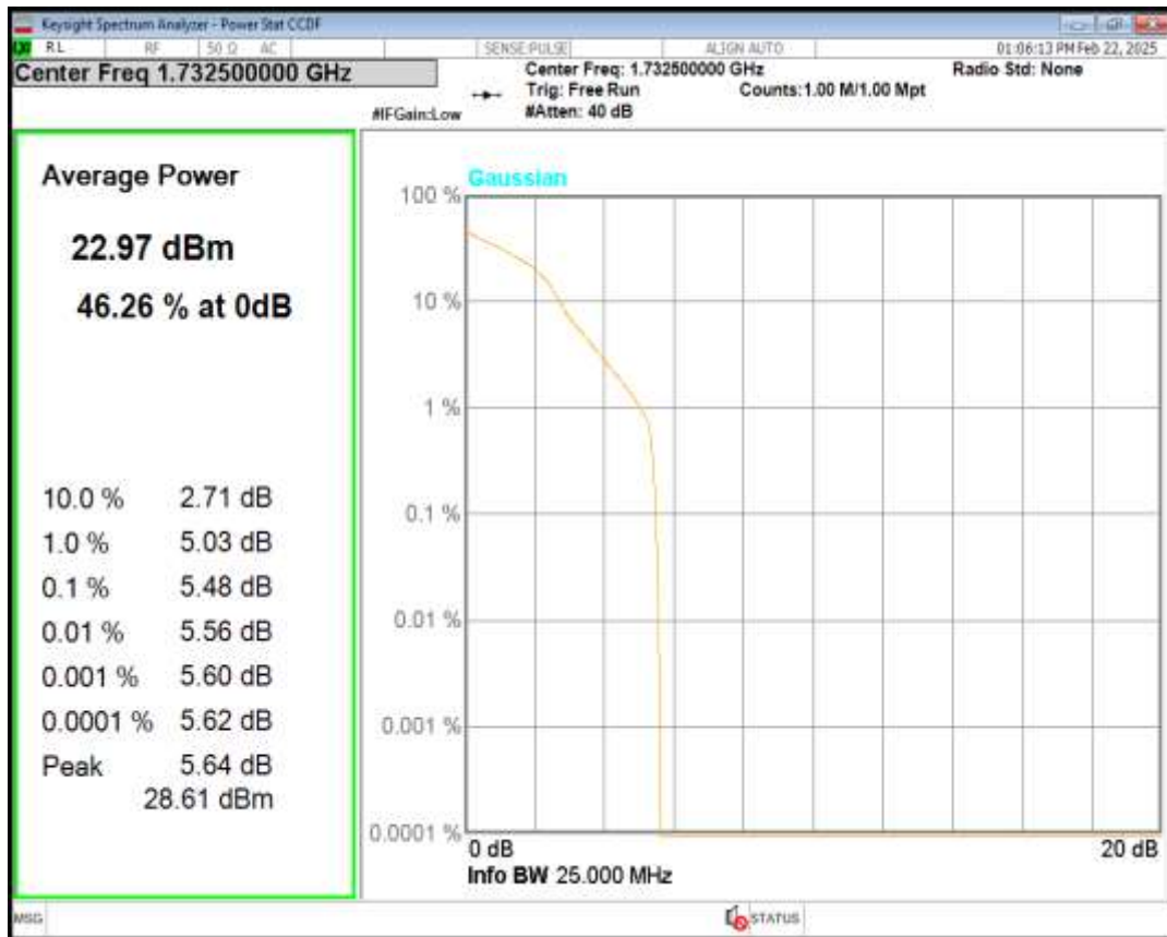
Band4 QPSK BW=15MHz Channel=20325 RB Size=1 Position=#0
