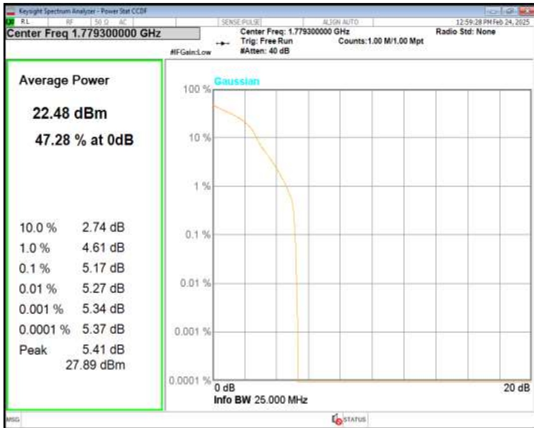
Band66 QPSK BW=3MHz Channel=131987 RB Size=1 Position=#0
