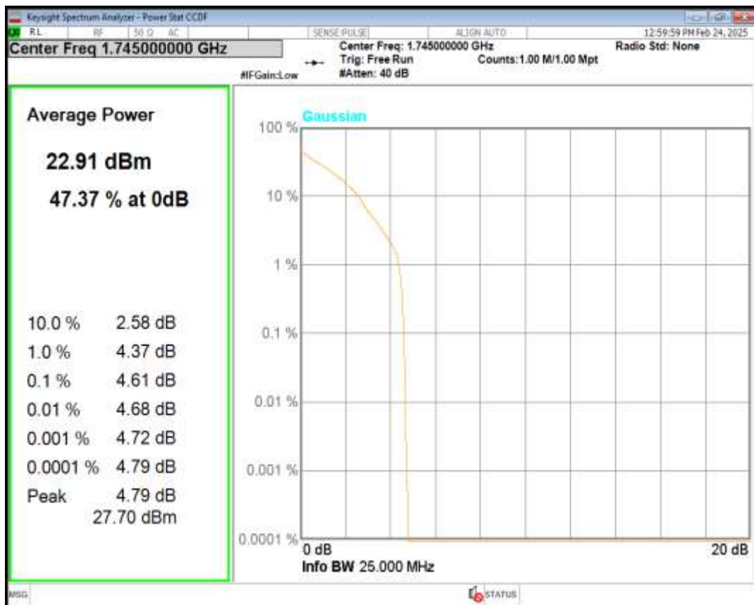
Band66 16QAM BW=5MHz Channel=132322 RB Size=1 Position=#0
