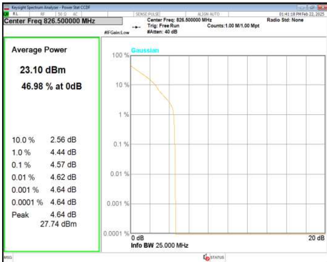
Band5 16QAM BW=5MHz Channel=20425 RB Size=1 Position=#0
