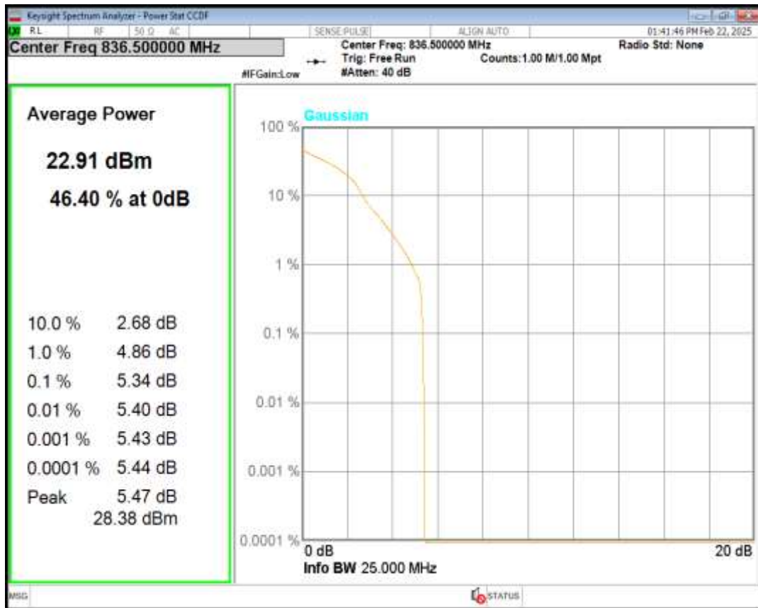
Band5 QPSK BW=10MHz Channel=20600 RB Size=1 Position=#0
