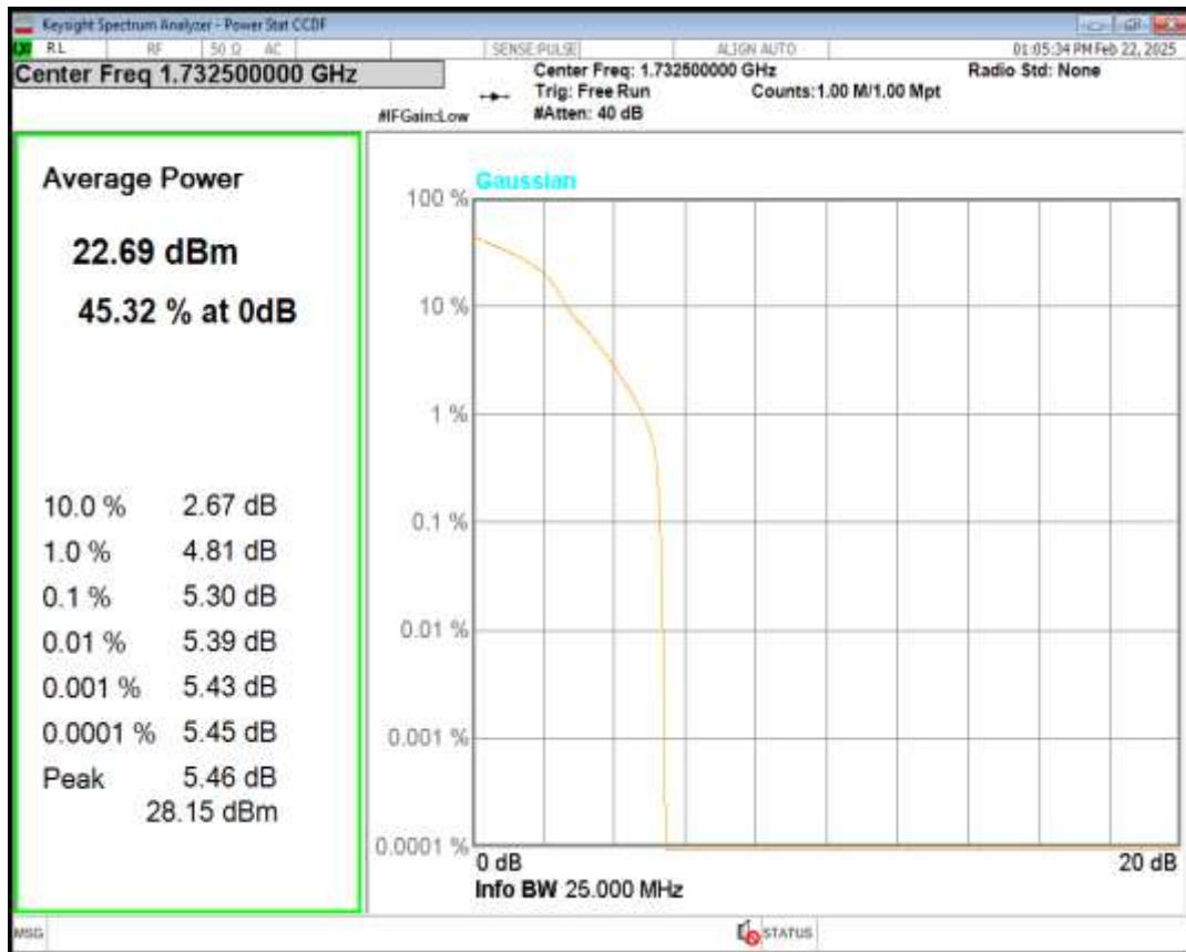
Band4 QPSK BW=5MHz Channel=20375 RB Size=1 Position=#0
