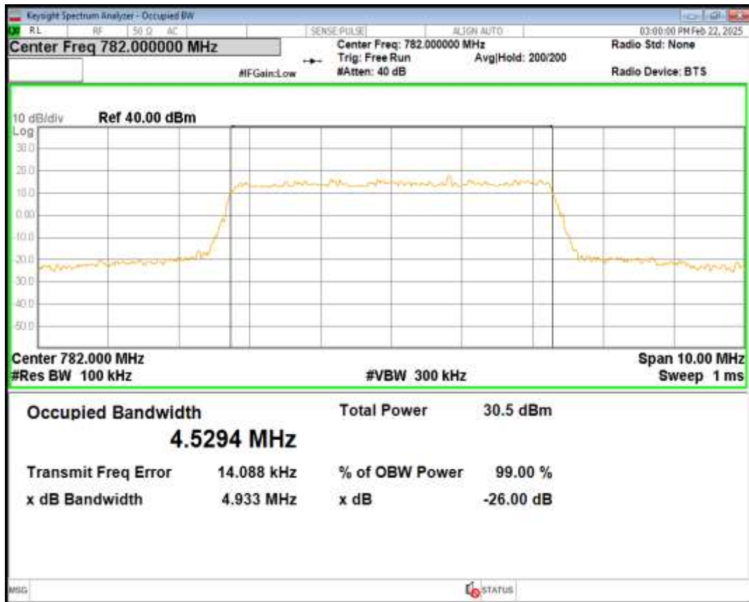
Band13 16QAM BW=5MHz Channel=23230 RB Size=25 Position=#0
