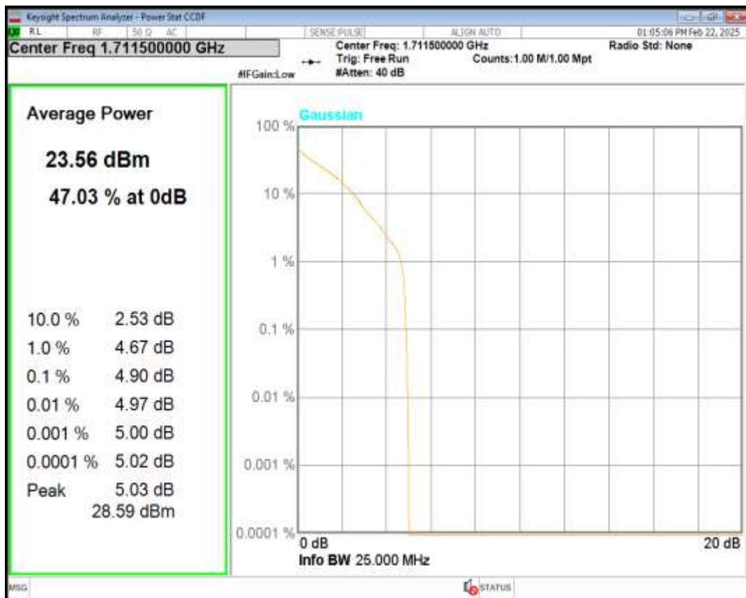
Band4 16QAM BW=3MHz Channel=19965 RB Size=1 Position=#0
