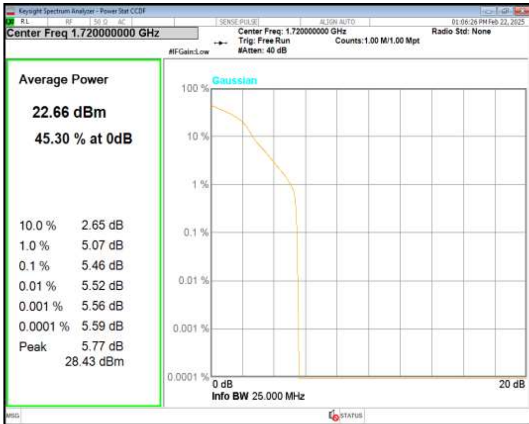
Band4 QPSK BW=20MHz Channel=20175 RB Size=1 Position=#0
