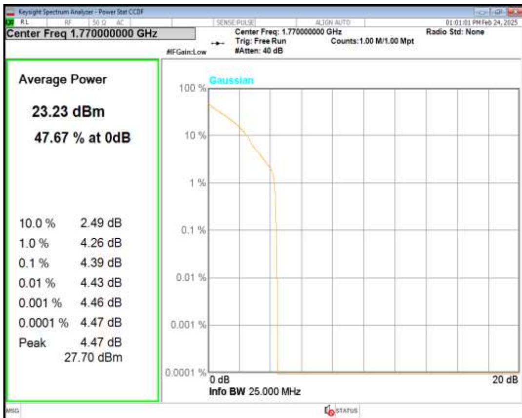
Band66 16QAM BW=20MHz Channel=132572 RB Size=1 Position=#0
