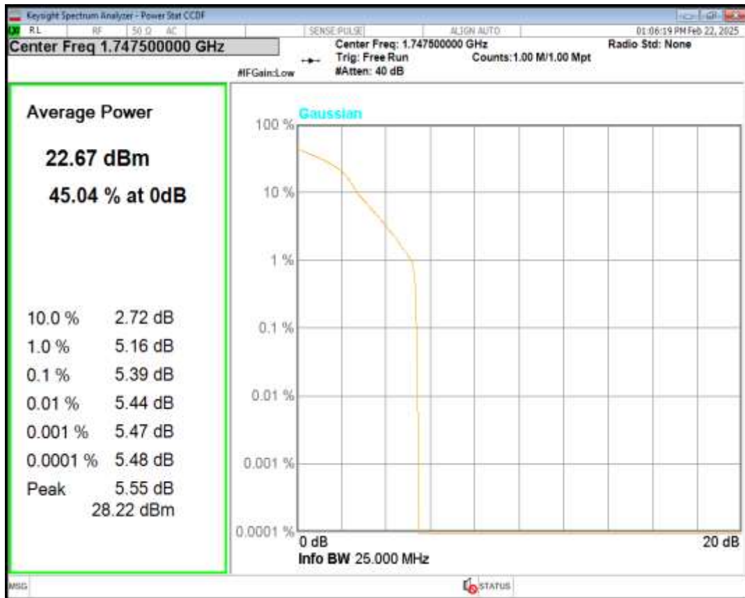
Band4 QPSK BW=20MHz Channel=20050 RB Size=1 Position=#0
