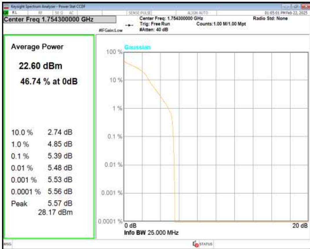
Band4 QPSK BW=3MHz Channel=19965 RB Size=1 Position=#0
