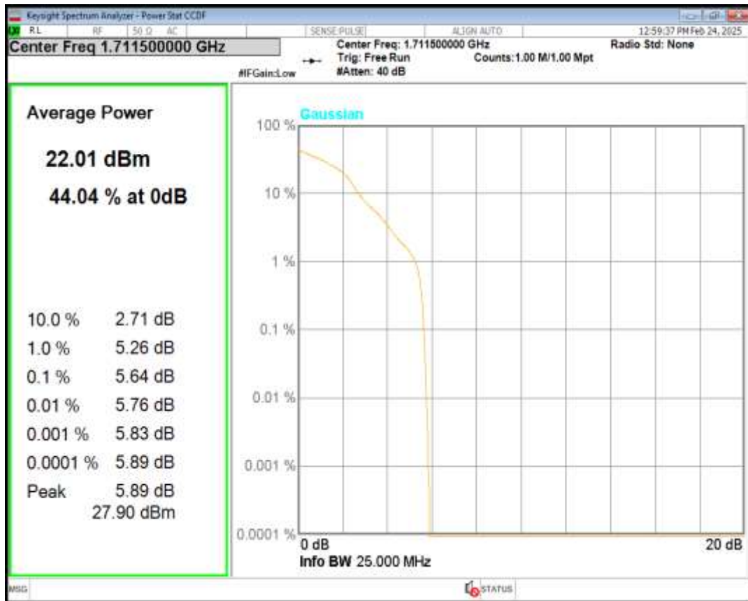
Band66 QPSK BW=3MHz Channel=132322 RB Size=1 Position=#0
