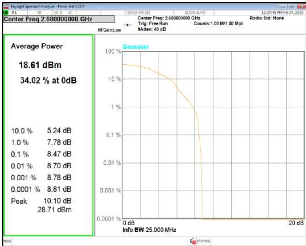
Band5 QPSK BW=1.4MHz Channel=20407 RB Size=1 Position=#0
