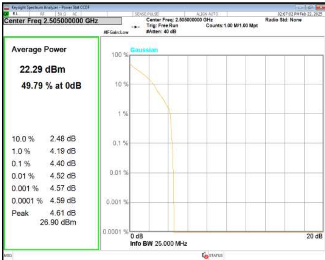
Band7 16QAM BW=10MHz Channel=20800 RB Size=1 Position=#0
