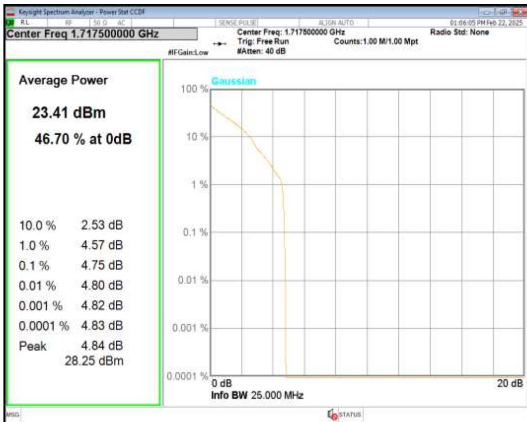
Band4 16QAM BW=15MHz Channel=20025 RB Size=1 Position=#0
