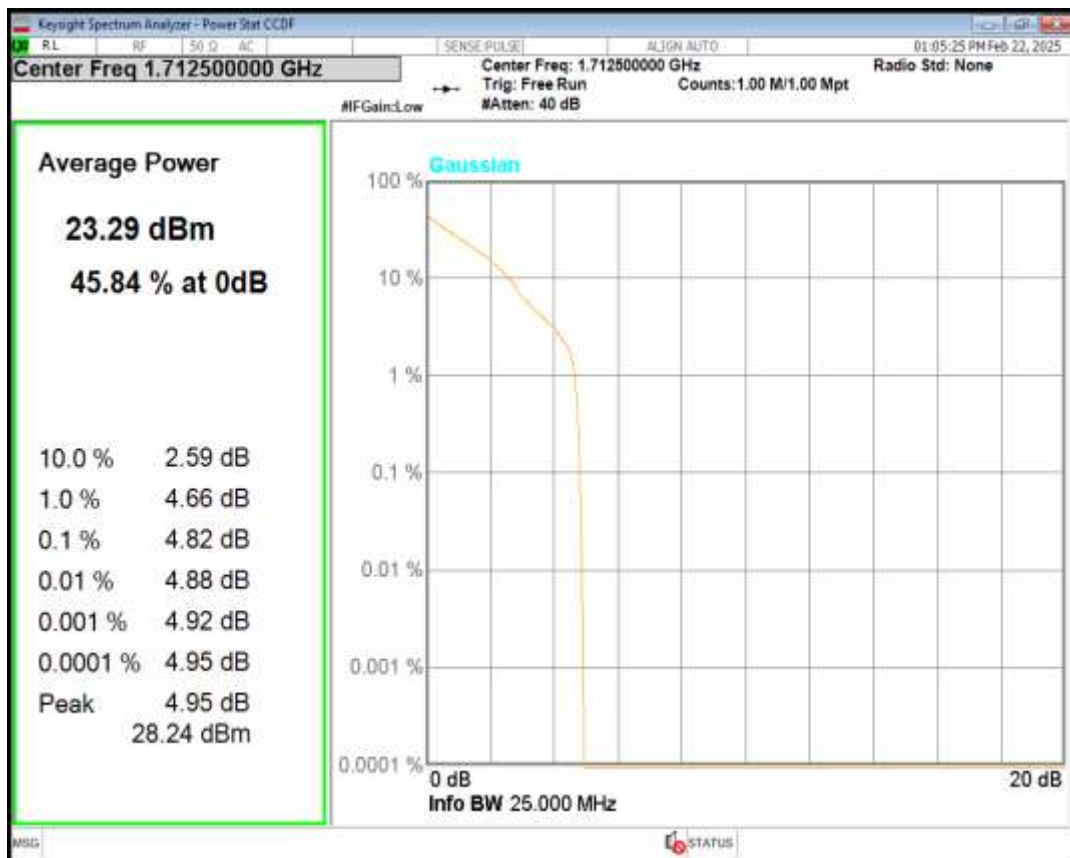
Band4 16QAM BW=5MHz Channel=19975 RB Size=1 Position=#0
