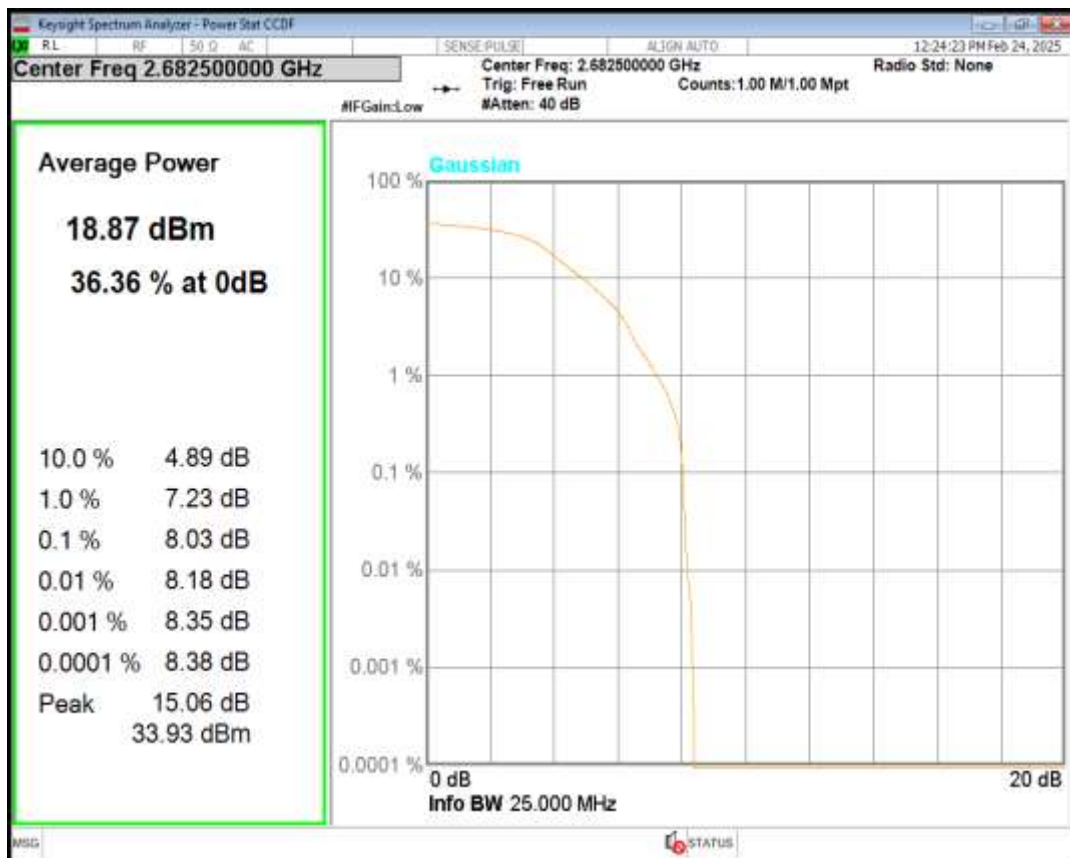
Band41 16QAM BW=15MHz Channel=41515 RB Size=1 Position=#0
