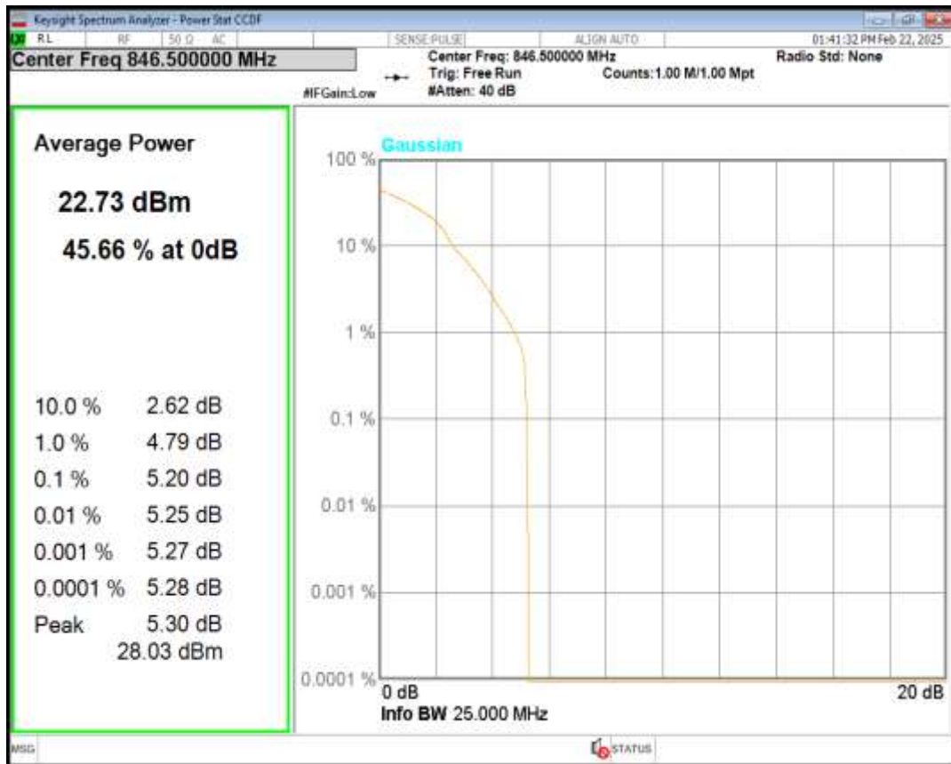
Band5 QPSK BW=10MHz Channel=20450 RB Size=1 Position=#0
