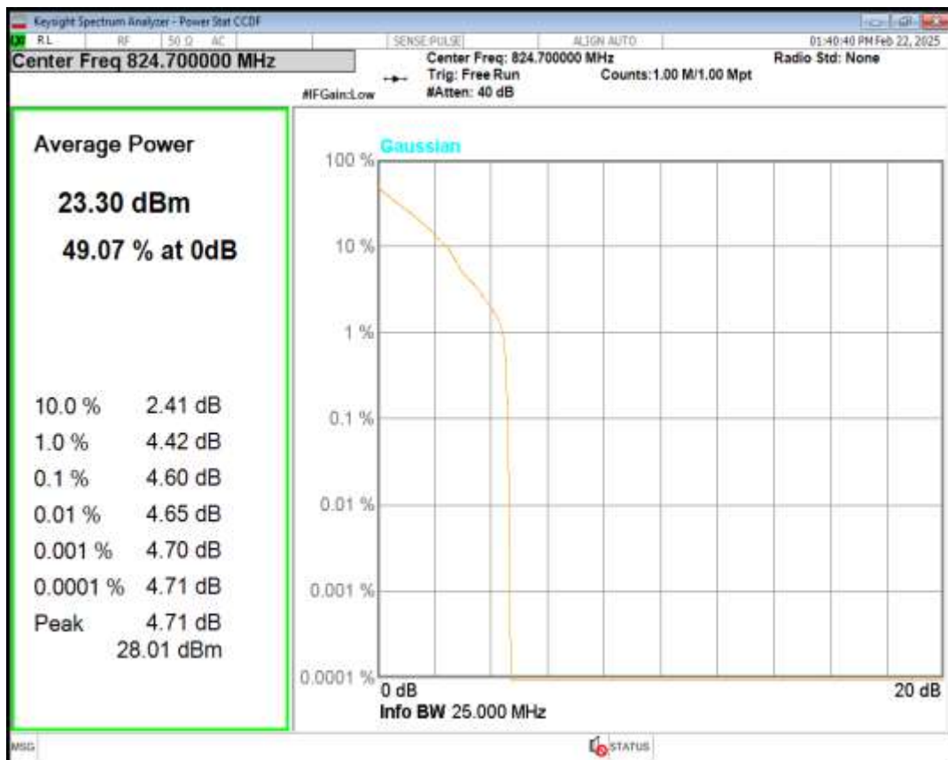
Band5 16QAM BW=1.4MHz Channel=20407 RB Size=1 Position=#0
