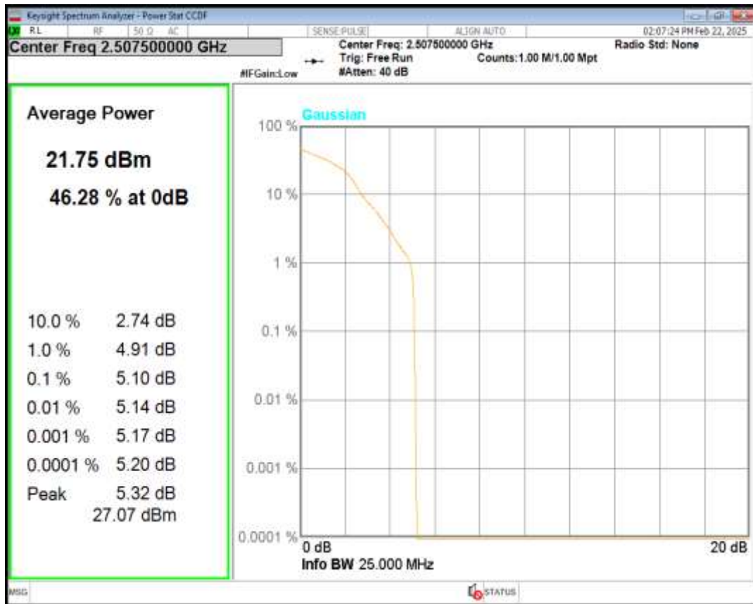
Band7 QPSK BW=15MHz Channel=21100 RB Size=1 Position=#0
