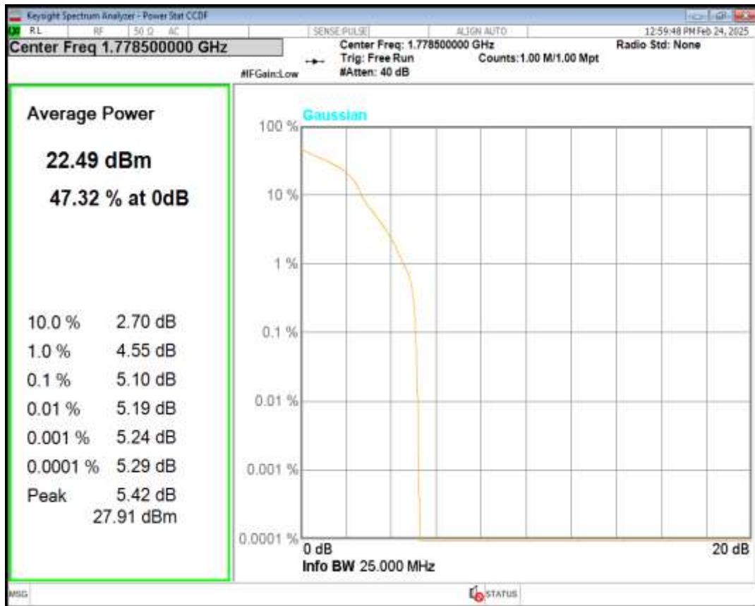
Band66 QPSK BW=5MHz Channel=131997 RB Size=1 Position=#0
