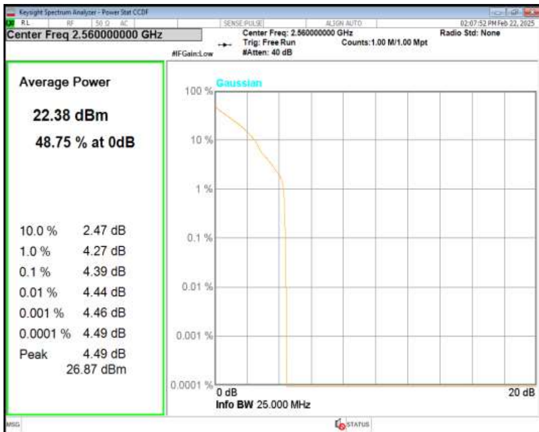
Band7 16QAM BW=20MHz Channel=21350 RB Size=1 Position=#0
