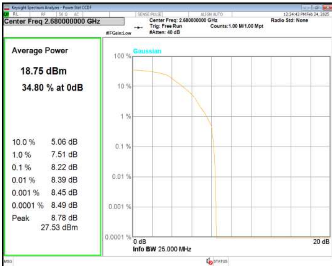
Band41 16QAM BW=20MHz Channel=41490 RB Size=1 Position=#0
