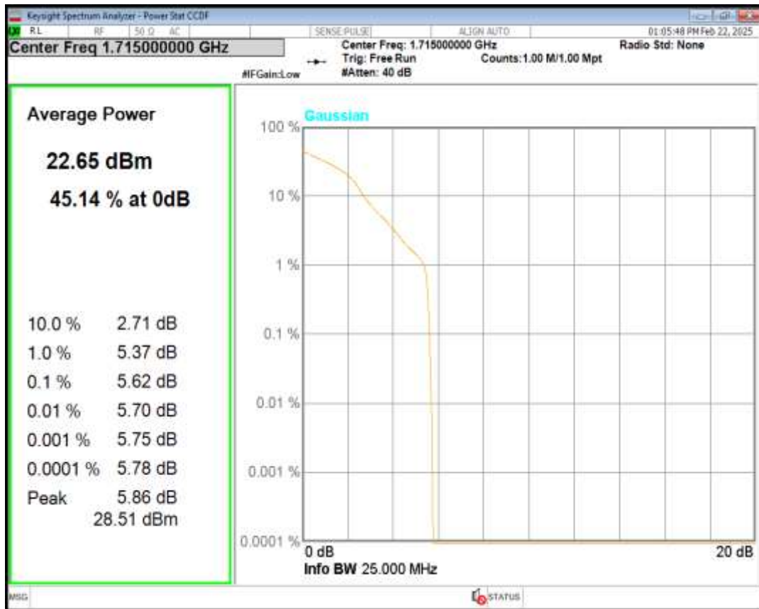
Band4 QPSK BW=10MHz Channel=20175 RB Size=1 Position=#0
