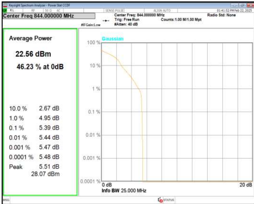
Band66 QPSK BW=1.4MHz Channel=131979 RB Size=1 Position=#0
