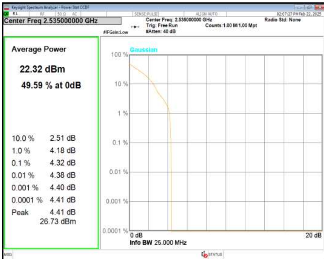
Band7 16QAM BW=15MHz Channel=21100 RB Size=1 Position=#0
