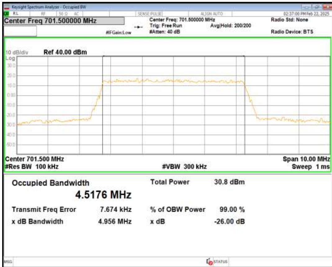
Band12 16QAM BW=5MHz Channel=23035 RB Size=25 Position=#0
