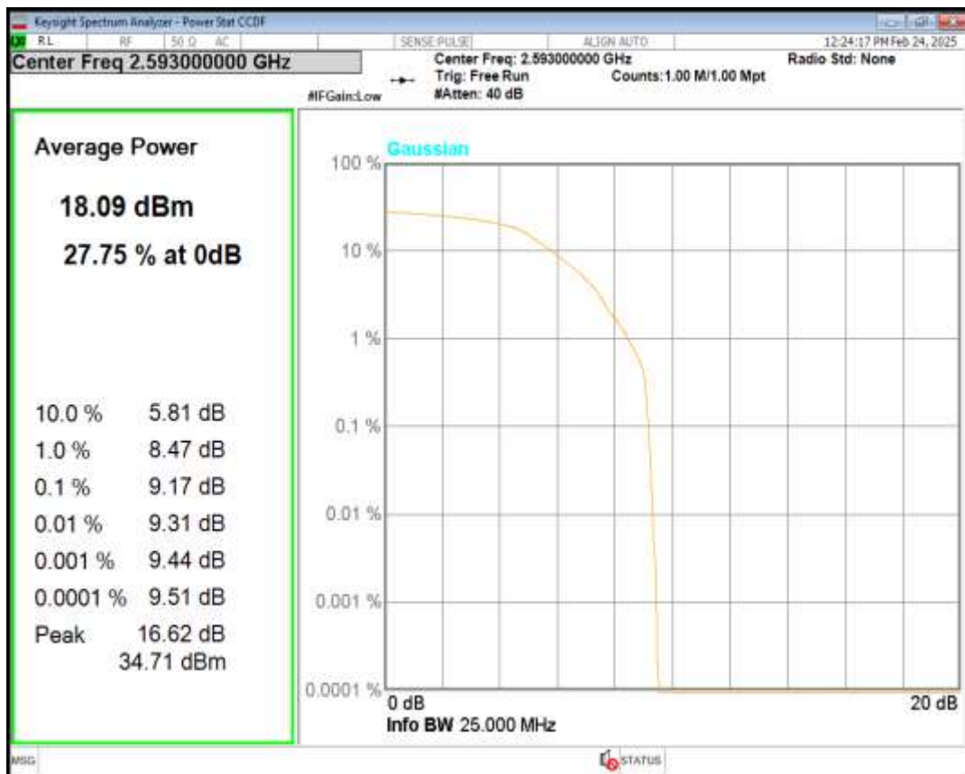
Band41 16QAM BW=15MHz Channel=40620 RB Size=1 Position=#0
