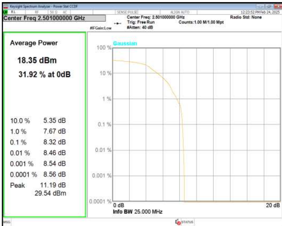
Band41 16QAM BW=10MHz Channel=39700 RB Size=1 Position=#0
