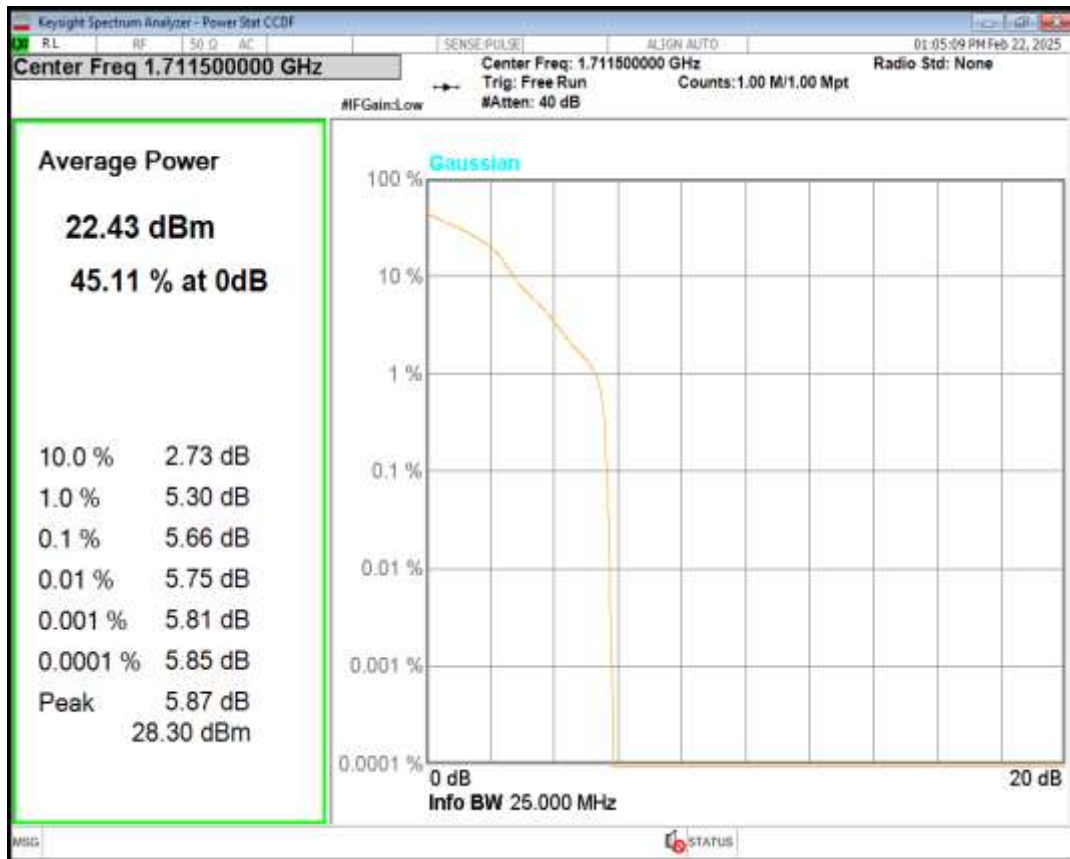
Band4 QPSK BW=3MHz Channel=20175 RB Size=1 Position=#0
