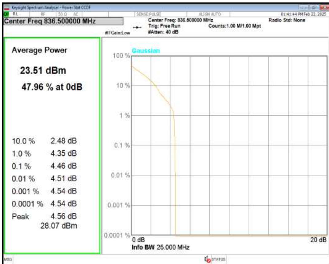
Band5 16QAM BW=10MHz Channel=20525 RB Size=1 Position=#0
