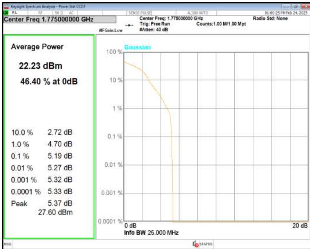
Band66 QPSK BW=15MHz Channel=132047 RB Size=1 Position=#0
