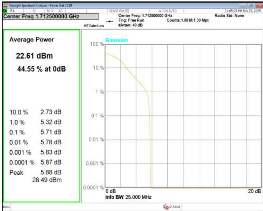
Band4 QPSK BW=5MHz Channel=20175 RB Size=1 Position=#0
