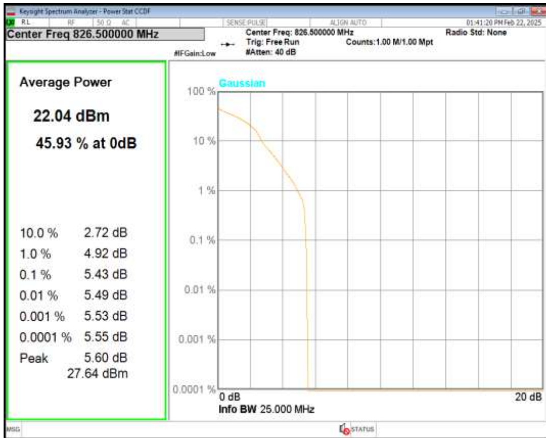
Band5 QPSK BW=5MHz Channel=20525 RB Size=1 Position=#0
