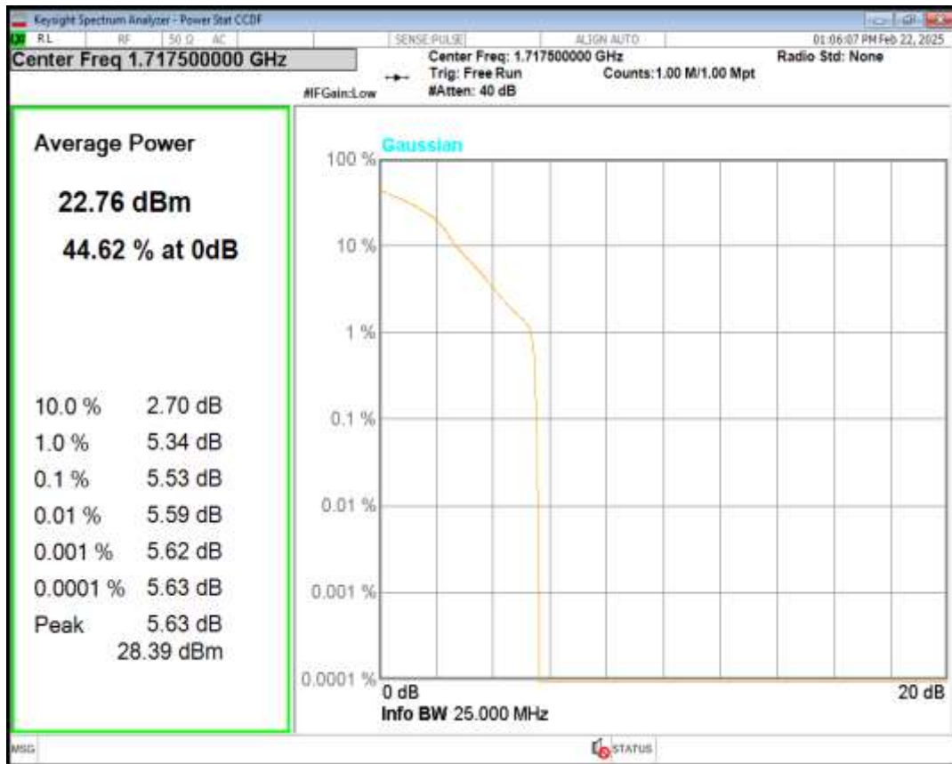
Band4 QPSK BW=15MHz Channel=20175 RB Size=1 Position=#0
