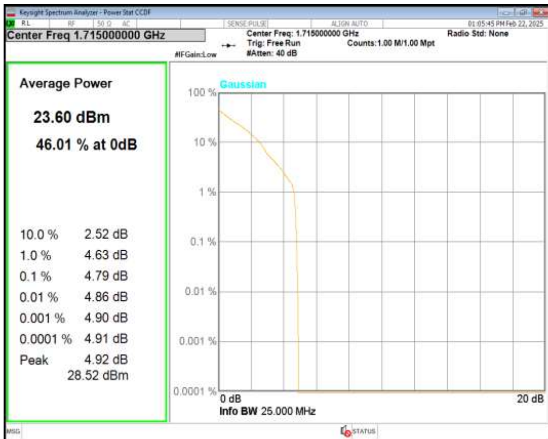
Band4 16QAM BW=10MHz Channel=20000 RB Size=1 Position=#0
