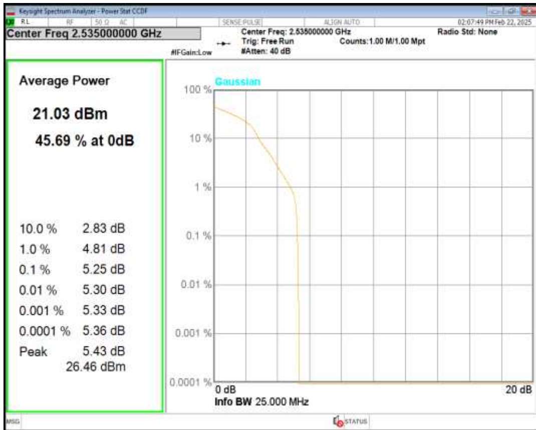
Band7 QPSK BW=20MHz Channel=21350 RB Size=1 Position=#0
