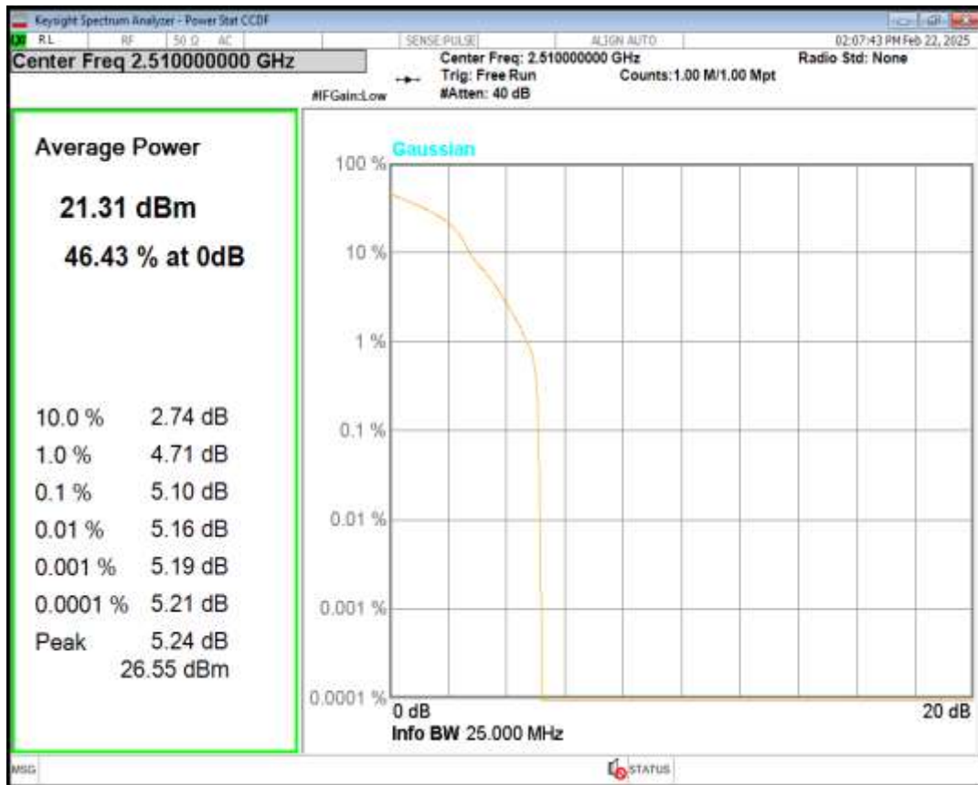
Band7 QPSK BW=20MHz Channel=21100 RB Size=1 Position=#0
