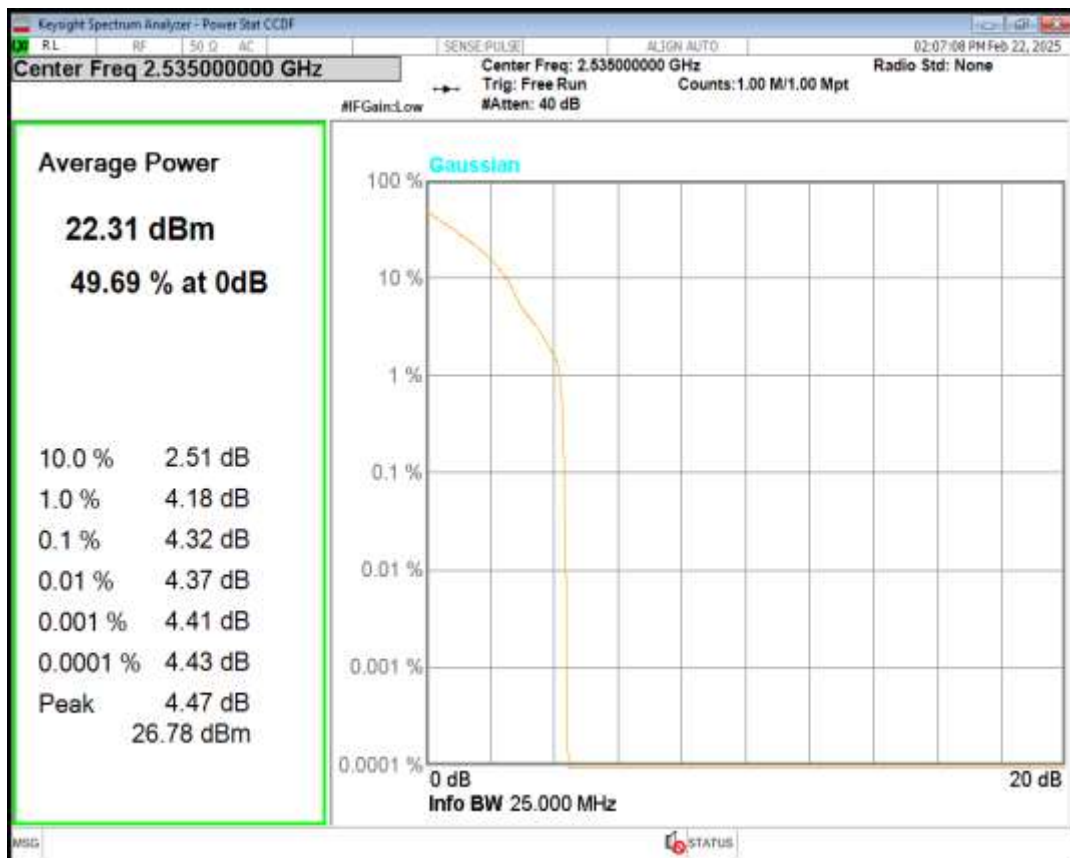
Band7 16QAM BW=10MHz Channel=21100 RB Size=1 Position=#0
