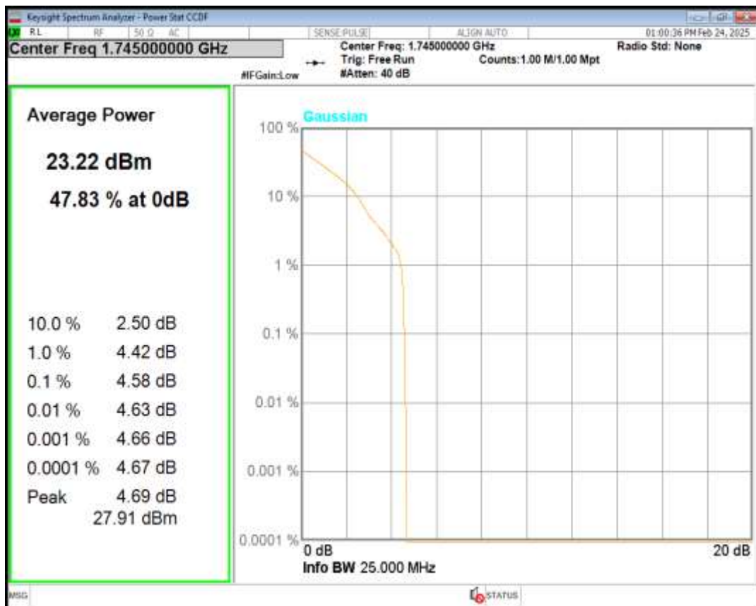
Band66 16QAM BW=15MHz Channel=132322 RB Size=1 Position=#0
