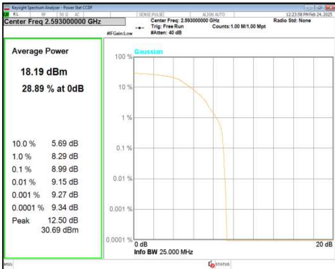
Band41 16QAM BW=10MHz Channel=40620 RB Size=1 Position=#0
