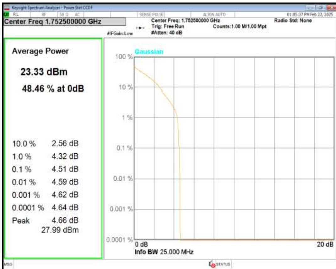
Band4 16QAM BW=5MHz Channel=20375 RB Size=1 Position=#0
