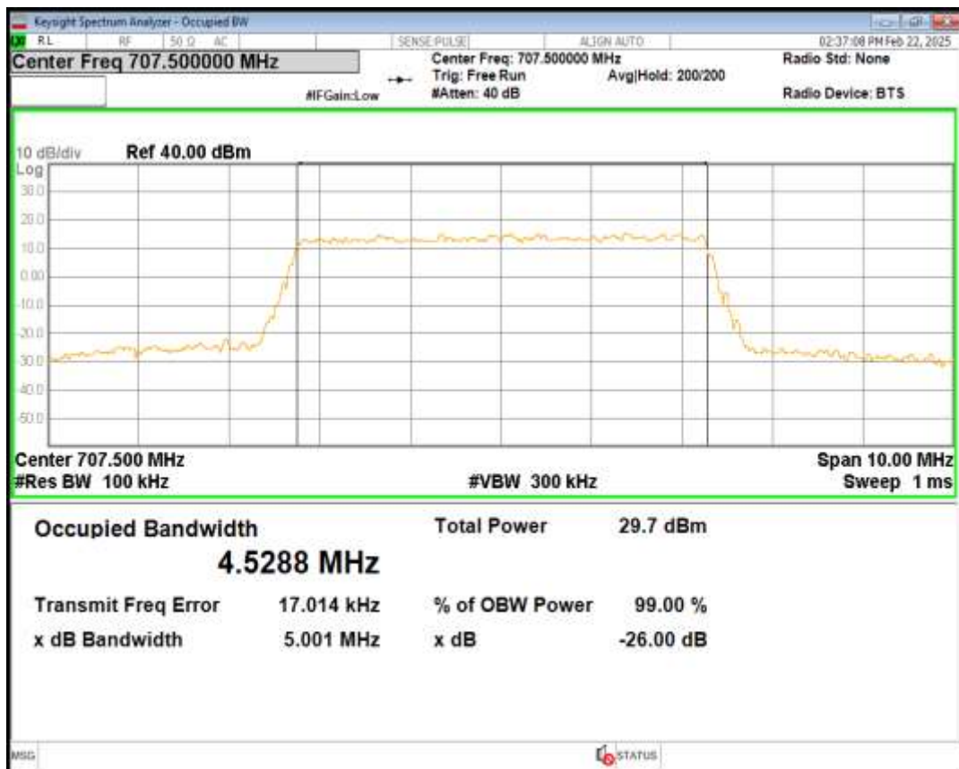
Band12 QPSK BW=5MHz Channel=23155 RB Size=25 Position=#0
