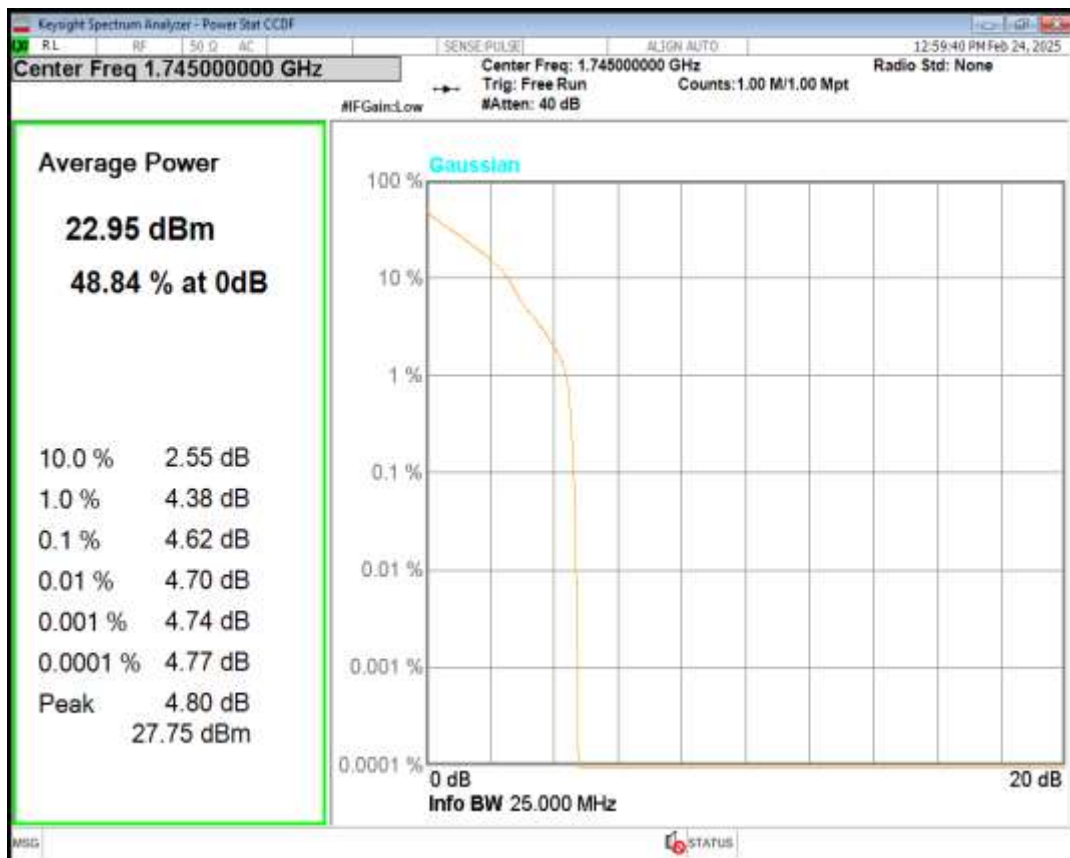
Band66 16QAM BW=3MHz Channel=132322 RB Size=1 Position=#0
