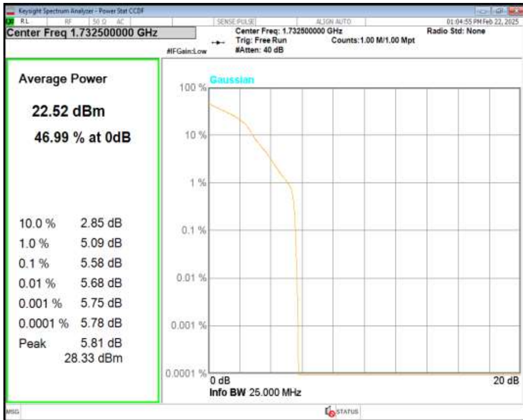
Band4 QPSK BW=1.4MHz Channel=20393 RB Size=1 Position=#0
