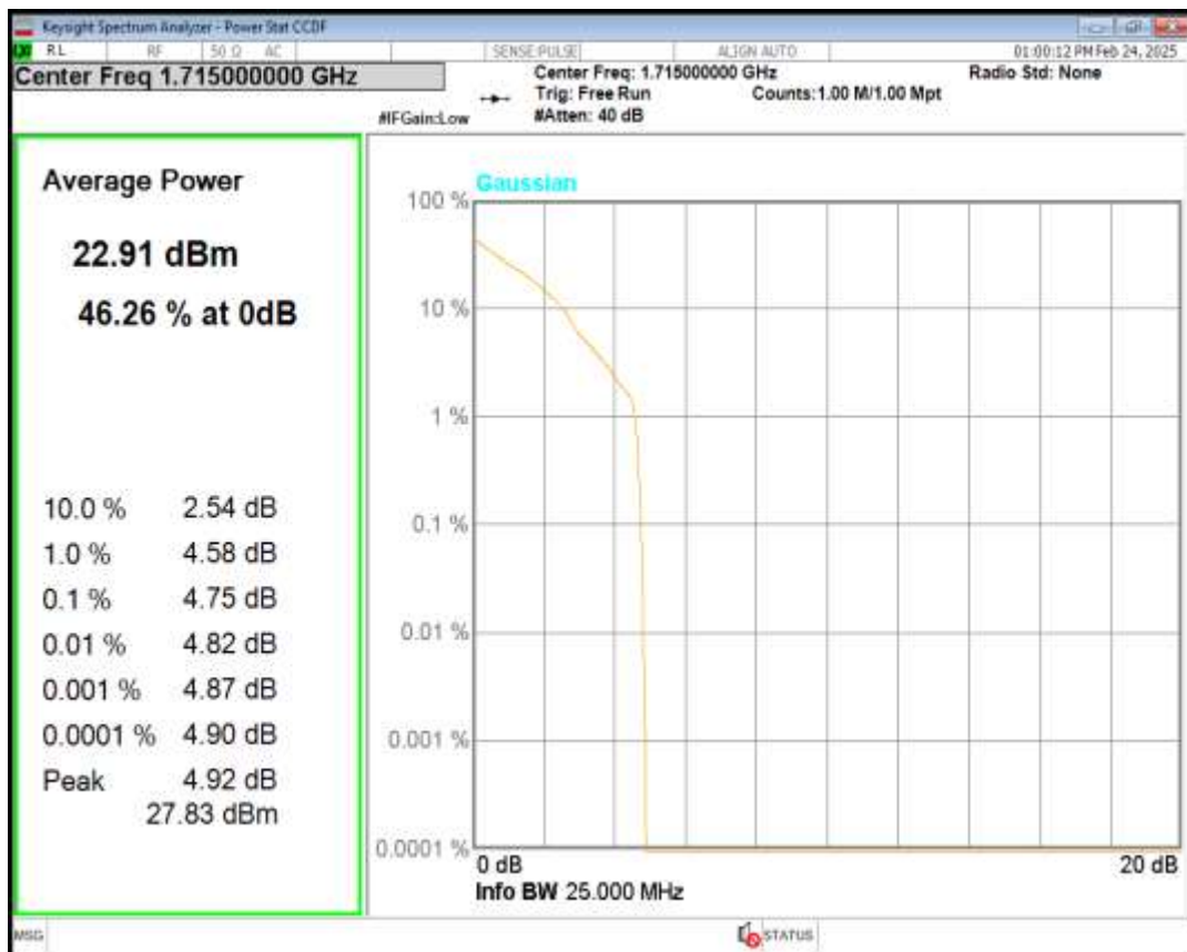
Band66 16QAM BW=10MHz Channel=132022 RB Size=1 Position=#0
