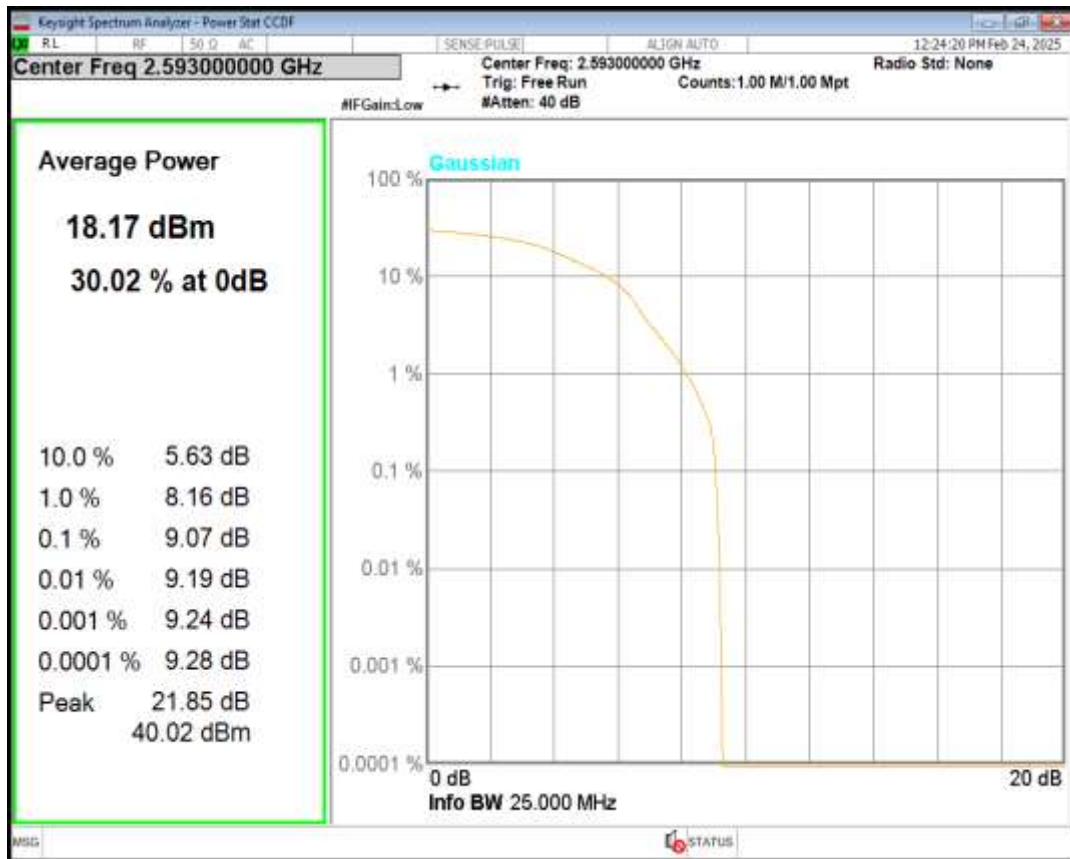
Band41 QPSK BW=15MHz Channel=41515 RB Size=1 Position=#0
