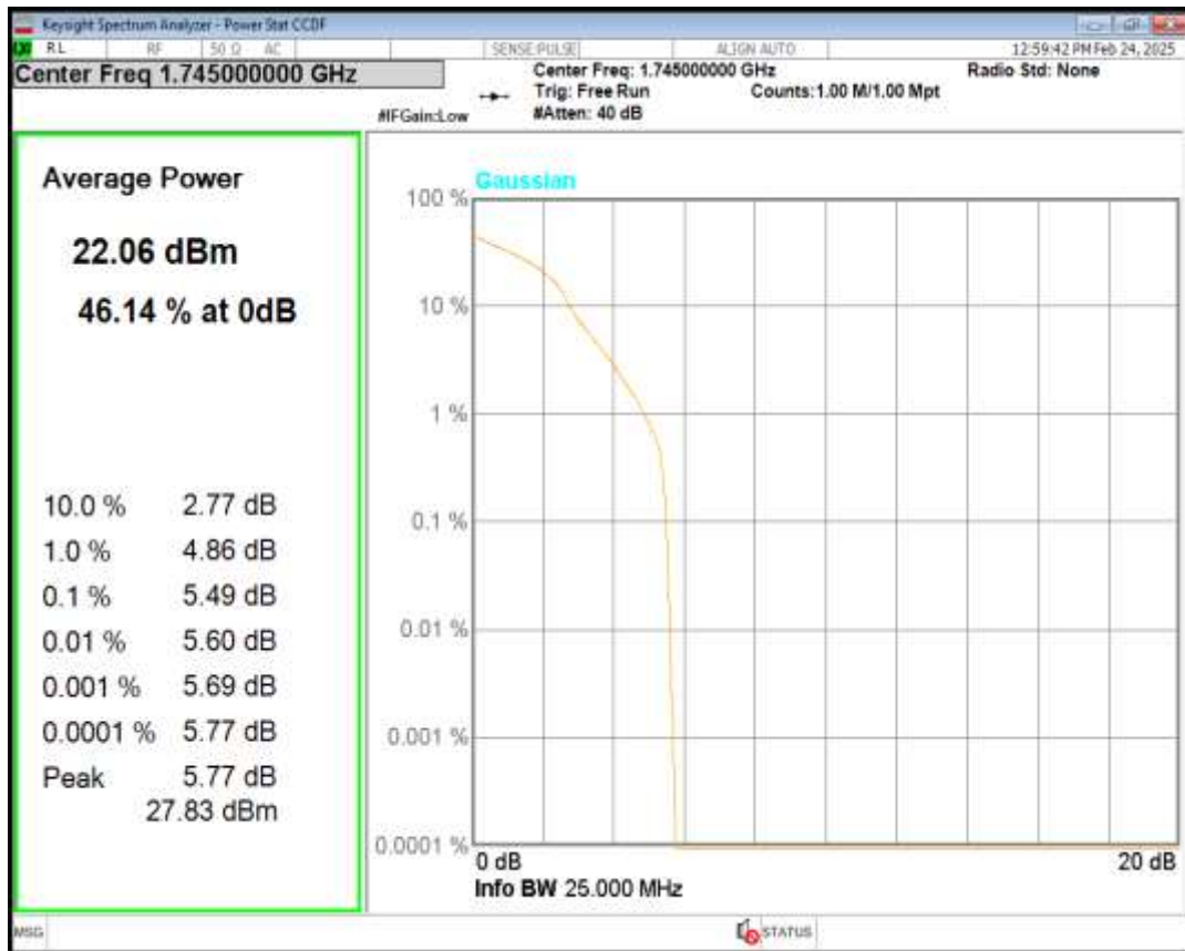
Band66 QPSK BW=3MHz Channel=132657 RB Size=1 Position=#0
