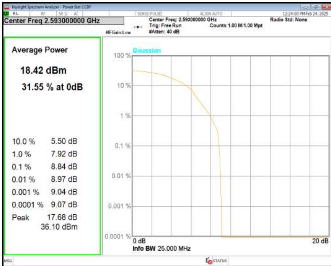
Band41 QPSK BW=10MHz Channel=41540 RB Size=1 Position=#0
