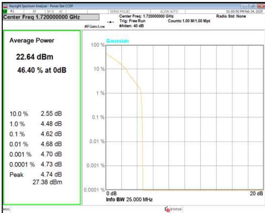
Band66 16QAM BW=20MHz Channel=132072 RB Size=1 Position=#0
