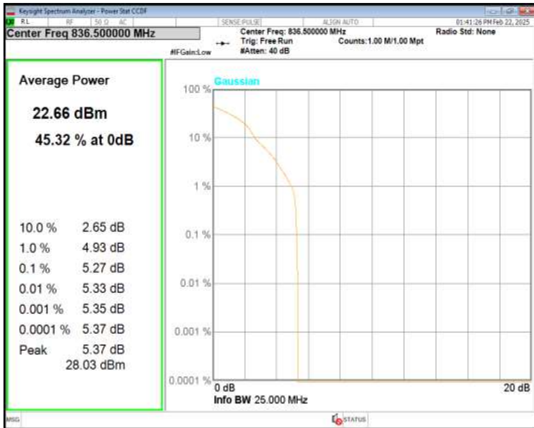
Band5 QPSK BW=5MHz Channel=20625 RB Size=1 Position=#0
