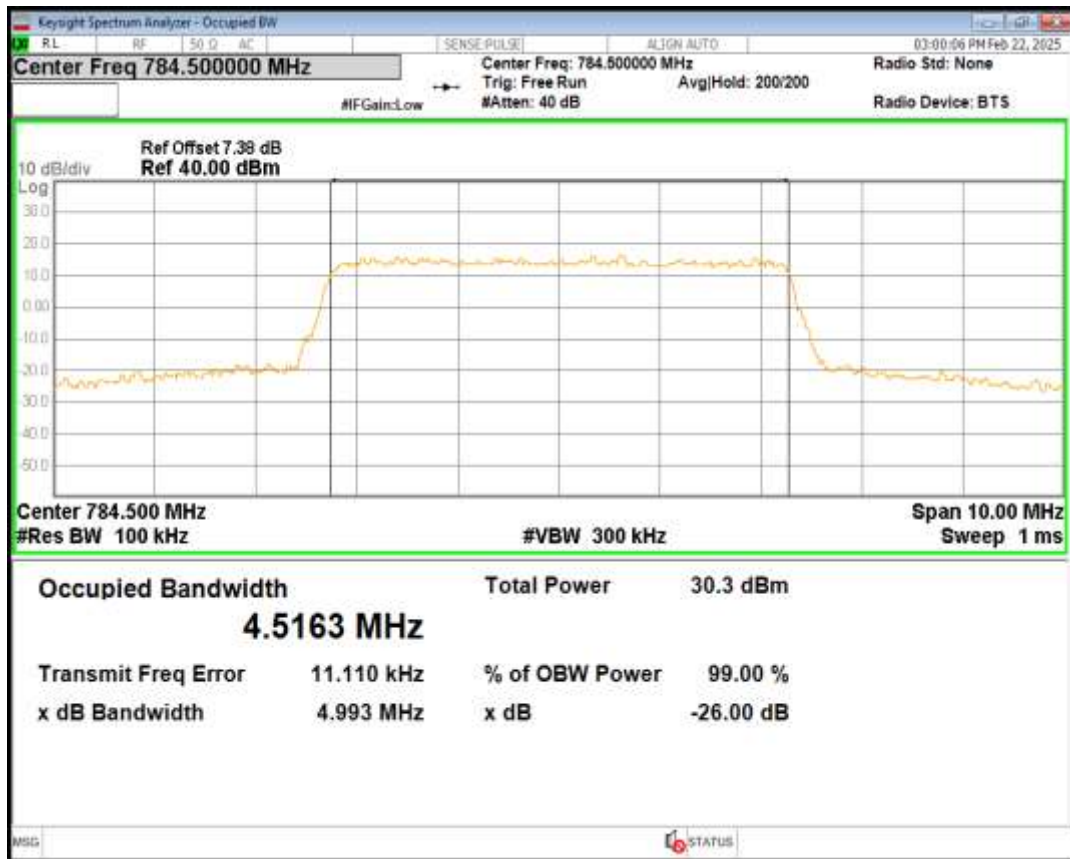
Band13 16QAM BW=5MHz Channel=23255 RB Size=25 Position=#0
