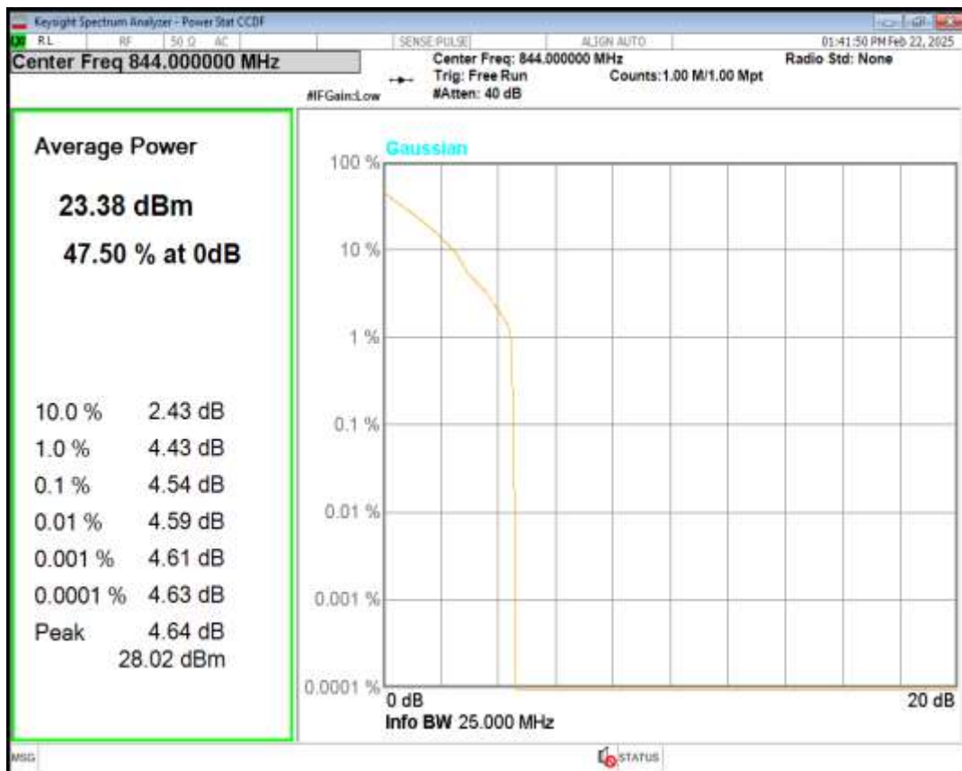
Band5 16QAM BW=10MHz Channel=20600 RB Size=1 Position=#0
