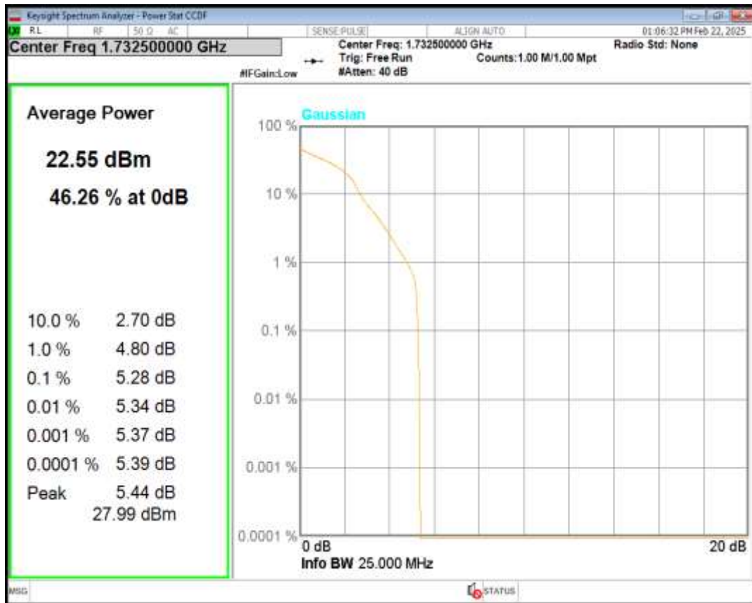
Band4 QPSK BW=20MHz Channel=20300 RB Size=1 Position=#0
