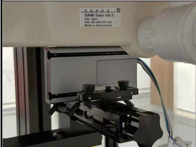
Left Side of EUT + Probe with 0 cm Gap
