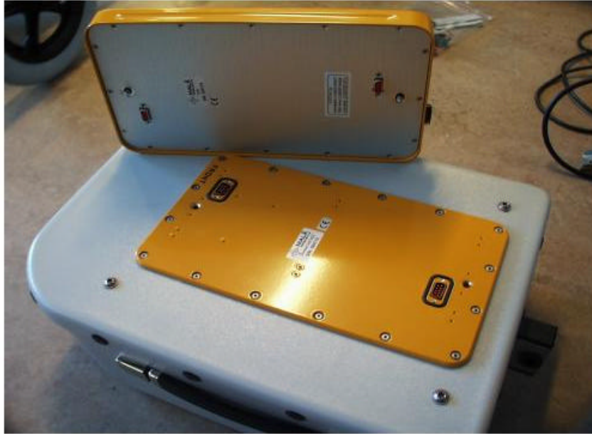
The bottom side of x3m/EasyLocator and top side of 500MHz antenna. Showing the D-sub connectors transferring dc-power and trig signals to the receiving and transmitting parts inside the antenna
