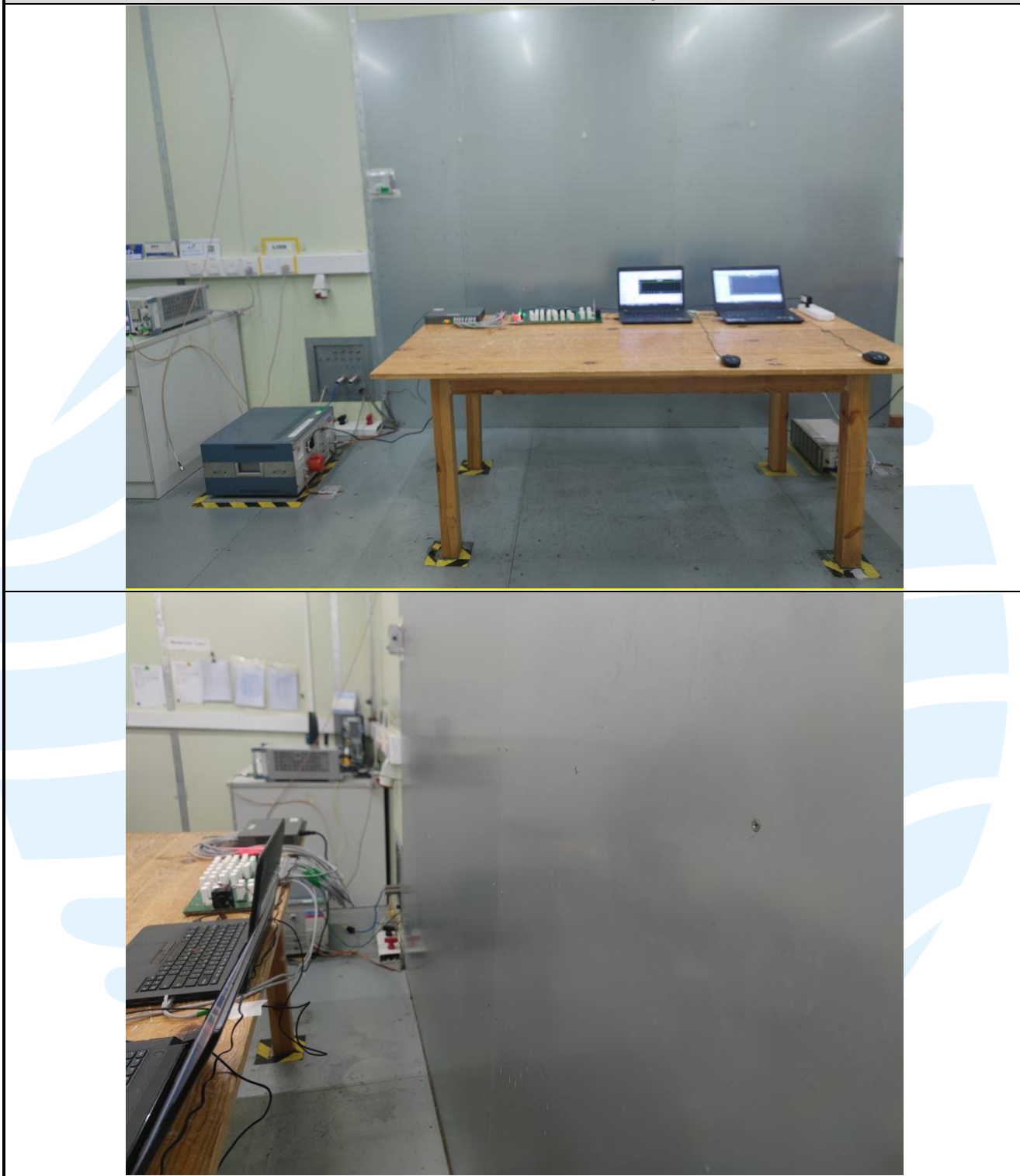
Conducted Emission Test Setup-3
