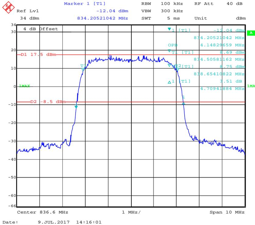
**99% Occupied Bandwidth & 26 dB Emissions Bandwidth for HSUPA (BPSK) Mode**
