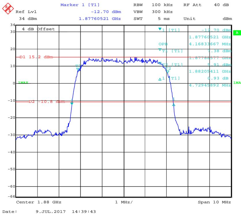
**99% Occupied Bandwidth & 26 dB Emissions Bandwidth for HSUPA (BPSK) Mode**
