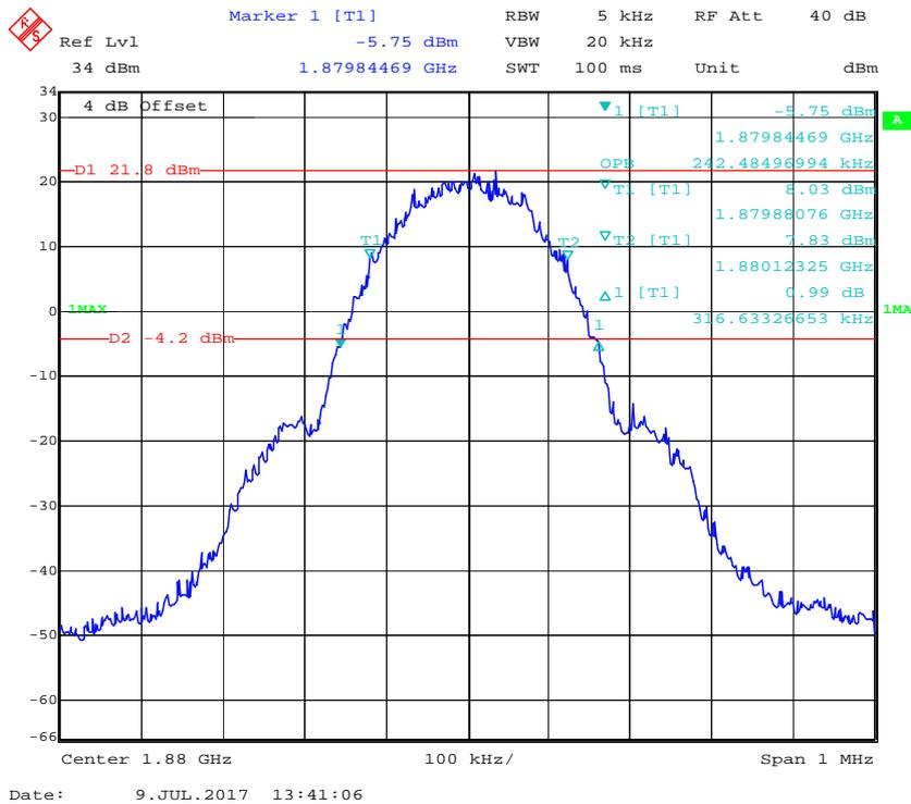
**26 dB Emissions & 99% Occupied Bandwidth for EGPRS (8PSK) Mode**
