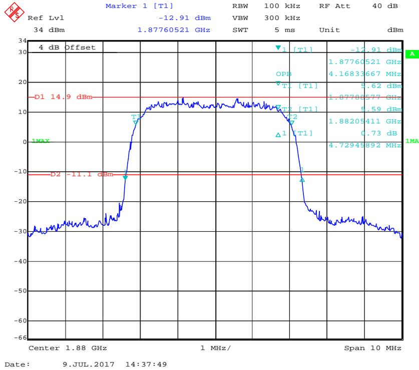
**99% Occupied Bandwidth & 26 dB Emissions Bandwidth for HSDPA (16QAM) Mode**
