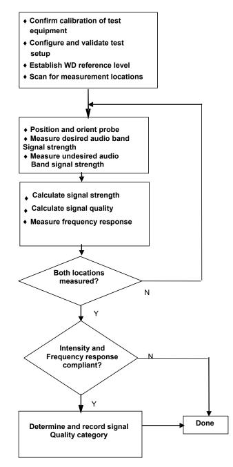
Figure 4-15 C63.19 T-Coil Signal Test Process
