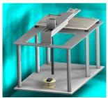
Figure 4-3 RF Near-Field Scanner
