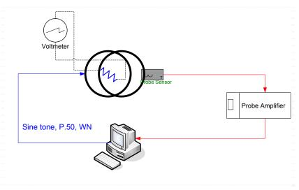
Figure 4-1 Validation Setup with Helmholtz Coil
