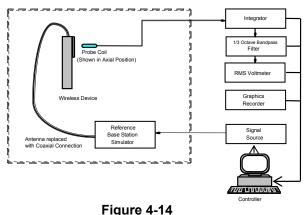
Figure 4-14 Audio Magnetic Field Test Setup
