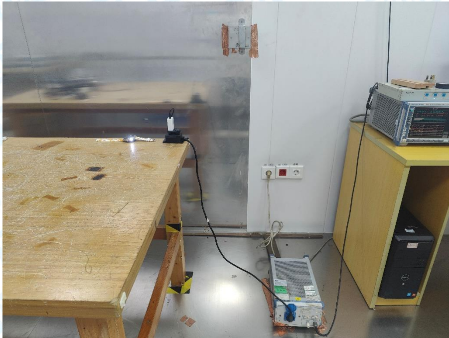
Photo of Setup for Radiated Emission (30MHz~1GHz)
