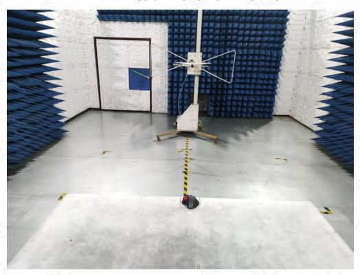
RADIATED EMISSION TEST SETUP ABOVE 1GHz
