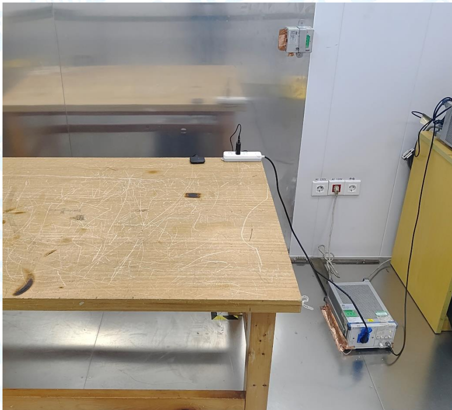
Photo of Setup for Conducted Emission
