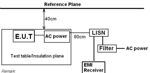
Remain. E.U.T: Equipment Under Test LISN: Line Impedence Stabilization Network Test table height=0.8m
