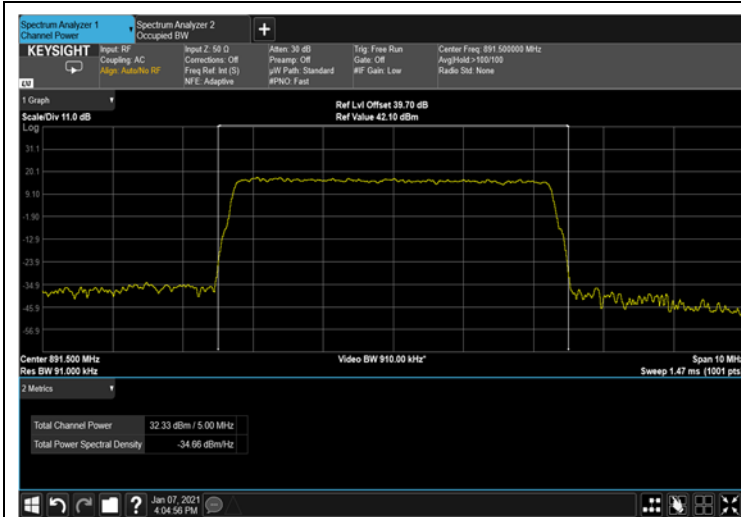
Figure 48: 256QAM 5MHz B.W.; 891.5MHz, 15kHz
