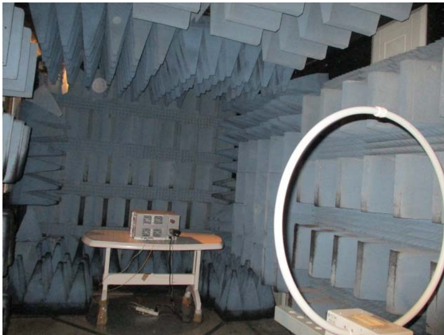
Figure 4. Radiated Emission Test 9kHz - 30MHz
