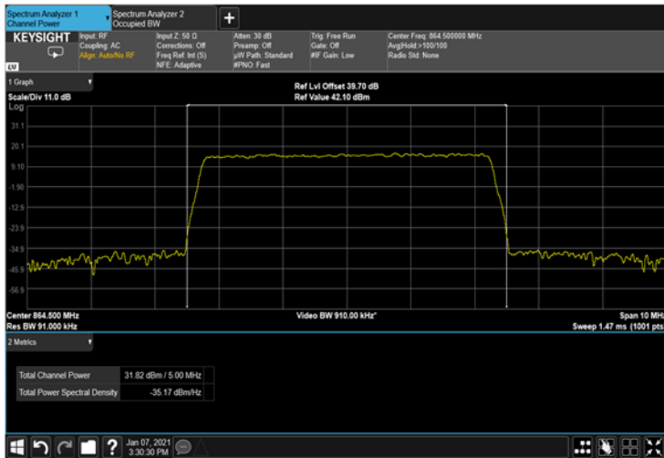
Figure 44: 256QAM 5MHz B.W.; 864.5MHz, 15kHz
