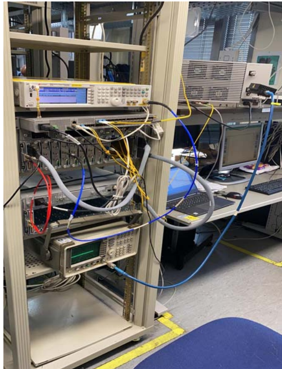
Figure 3. Conducted Emission From Antenna Port Tests
