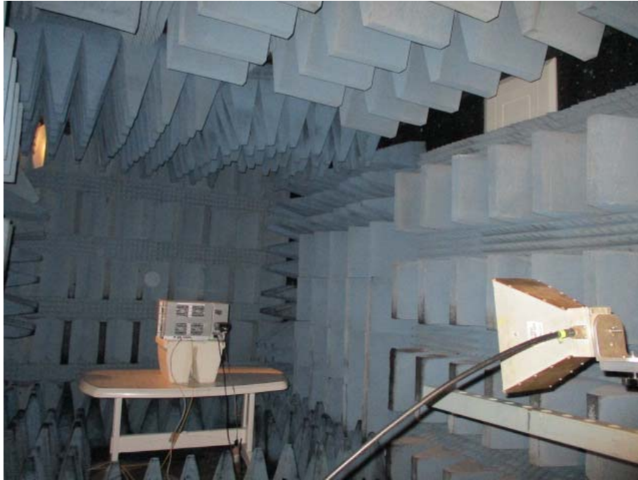
Figure 7. Radiated Emission Test 1.0 - 9.0GHz
