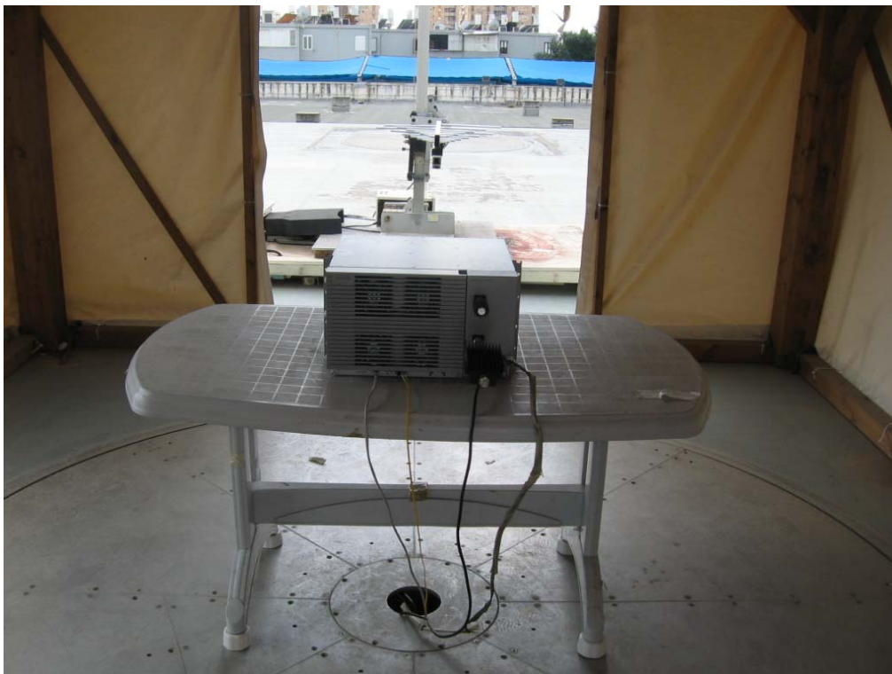
Figure 6. Radiated Emission Test 200 - 1000MHz
