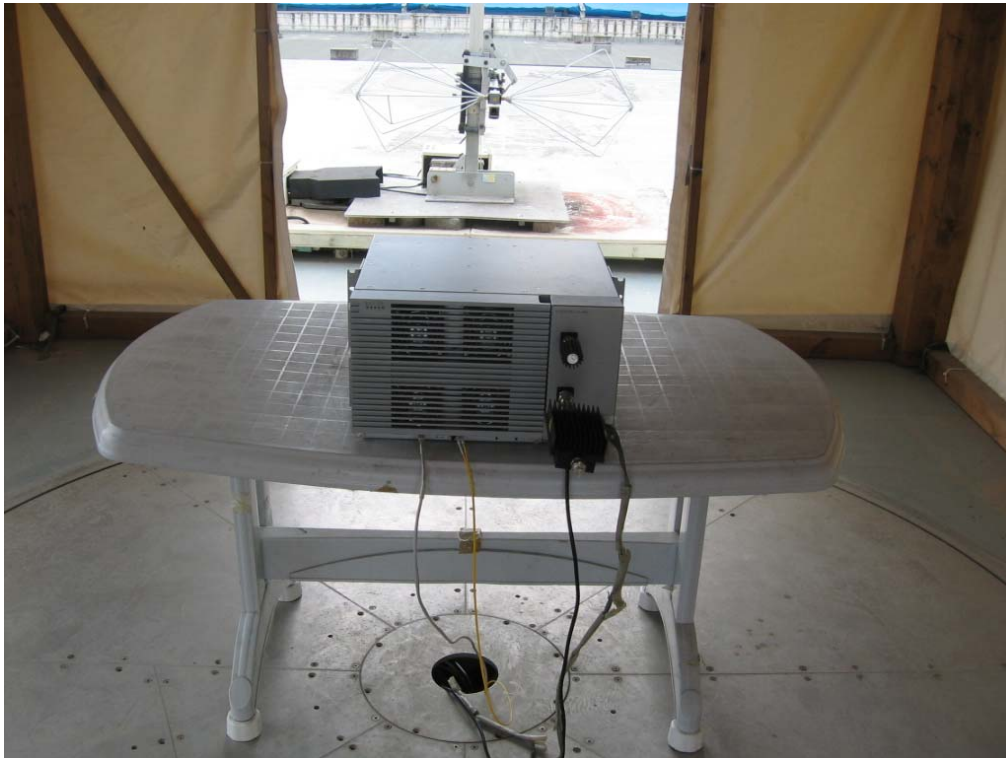
Figure 5. Radiated Emission Test 30 - 200 MHz
