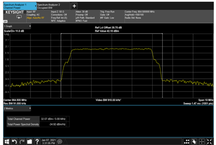
Figure 45: 256QAM 5MHz B.W.; 864.5MHz, 30kHz
