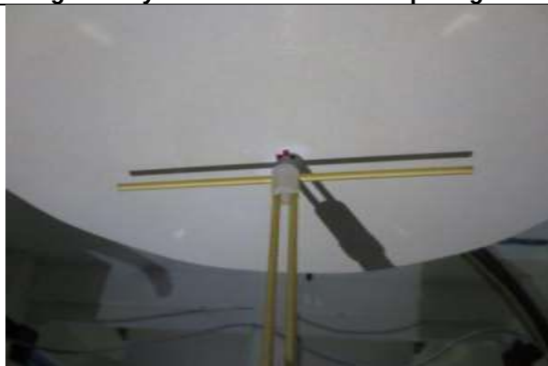
Fig.10.2 Photo of Dipole setup
