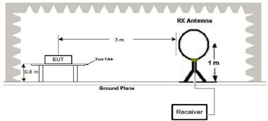
2. Radiated Emission Test-Up Frequency 30MHz~1GHz
