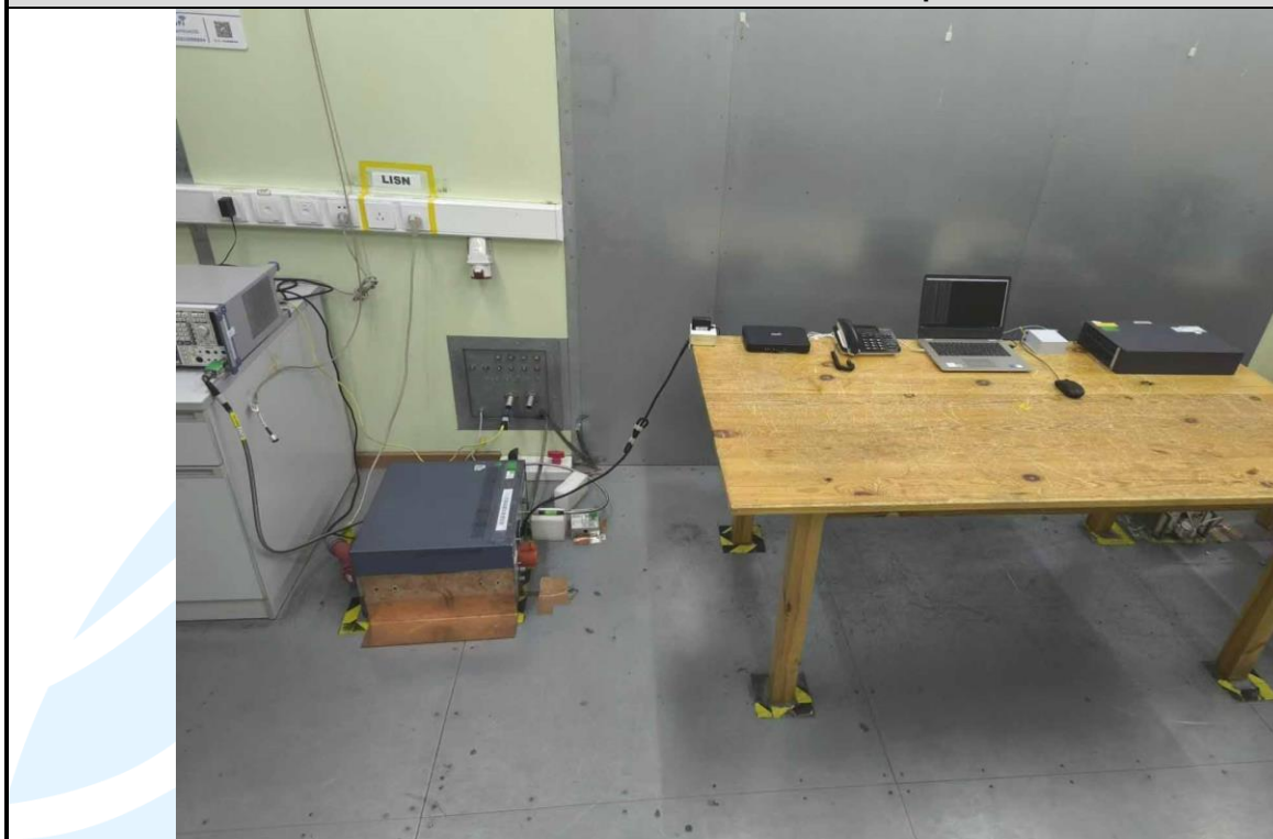
Conducted Emission Test Setup-3
