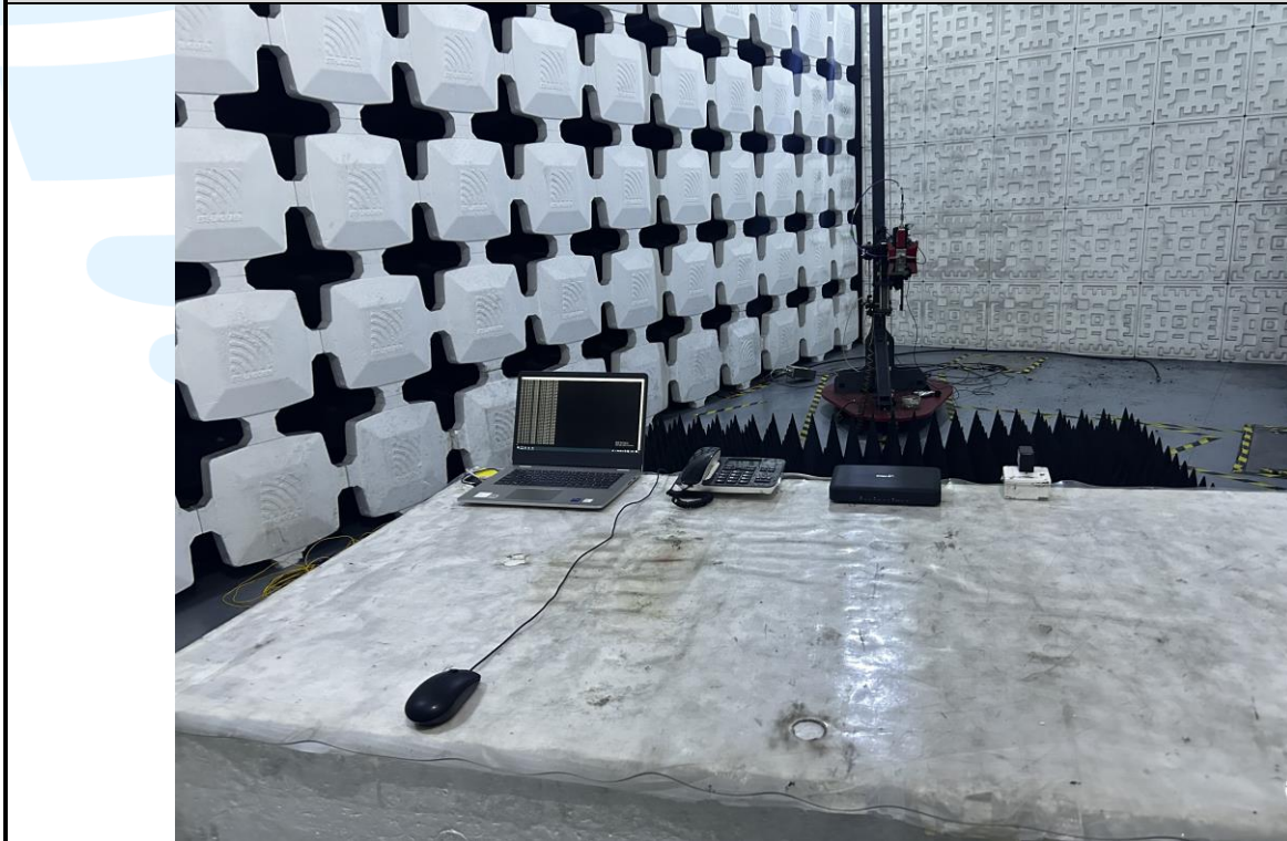
Radiated emission Test Setup-2 (Above 1 GHz)
