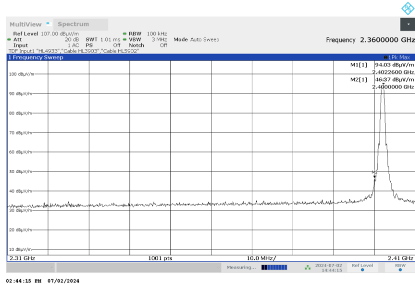
Plot 7.4.3 The highest emission level outside restricted bands at low carrier frequency
