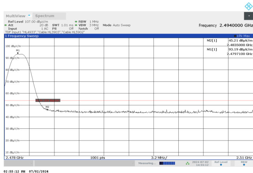
Plot 7.4.2 The highest band edge emission inside restricted bands at high carrier frequency
