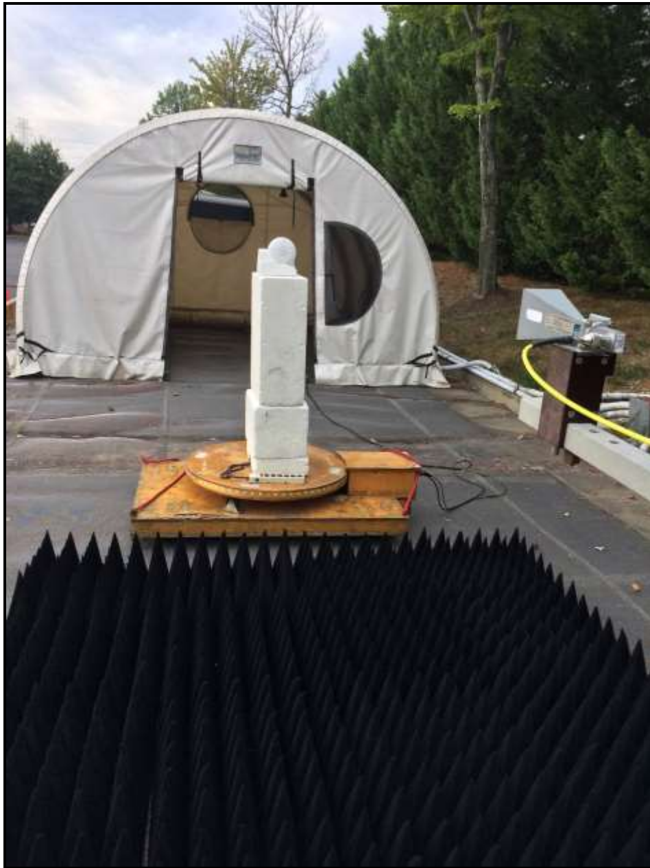
Photograph 3: Radiated Emissions Testing – Front View (Greater than 1 GHz)
