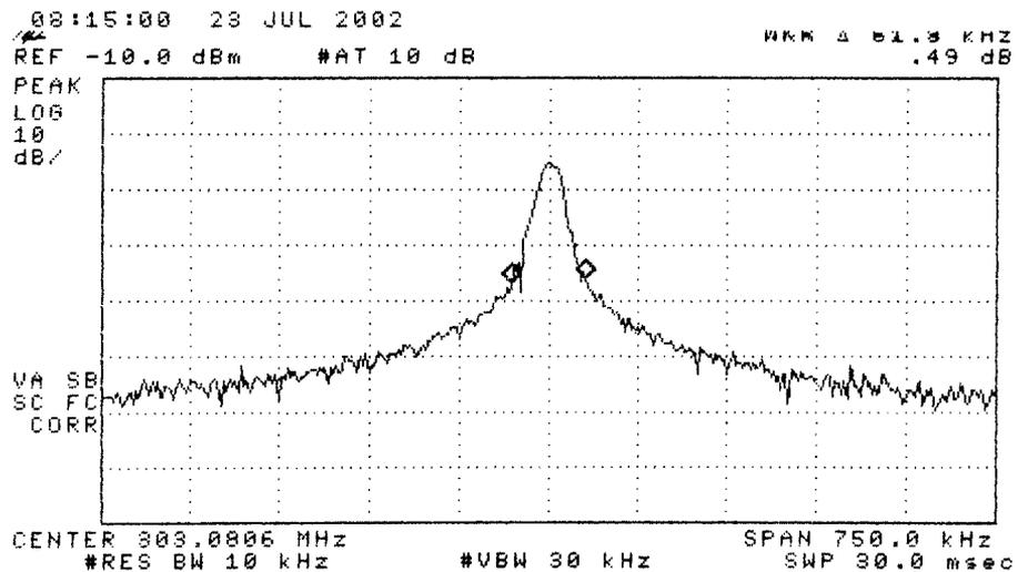
Figure 6.3. Measured bandwidth of the DUT (pulsed emission).
