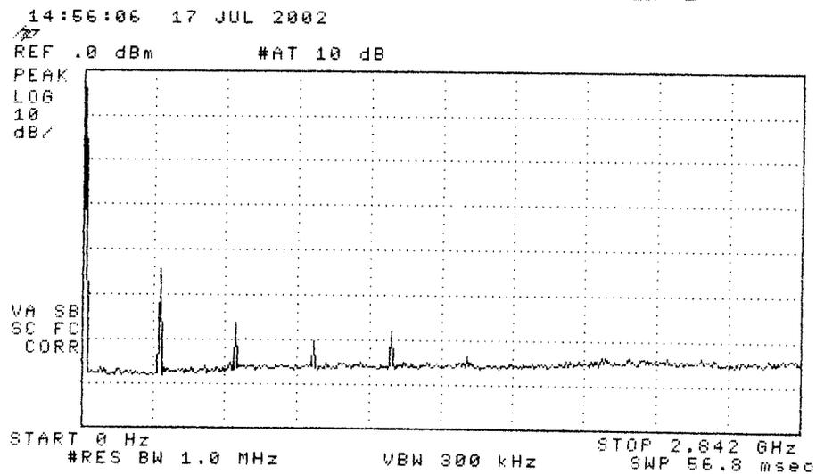
Figure 6.2. Emission spectrum of the DUT (pulsed emission).
