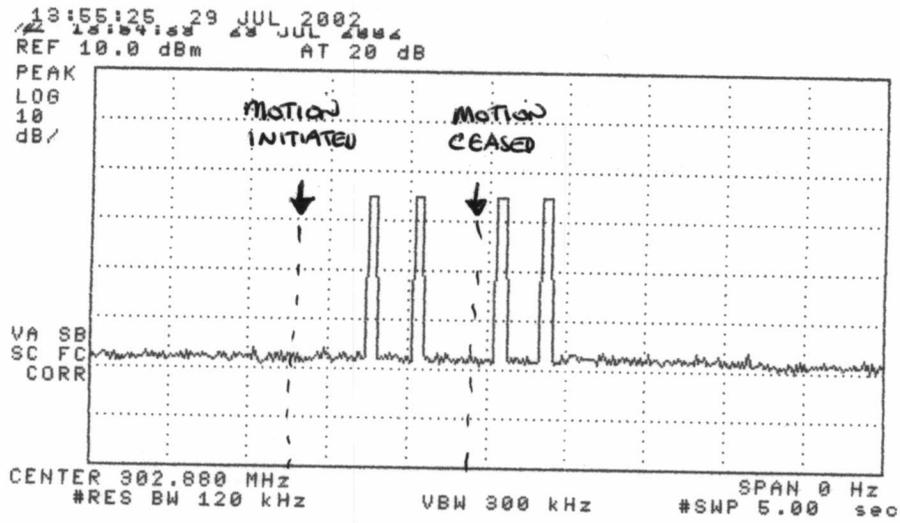
Figure 6.4. Transmitter 5 sec. transmission limit verification
