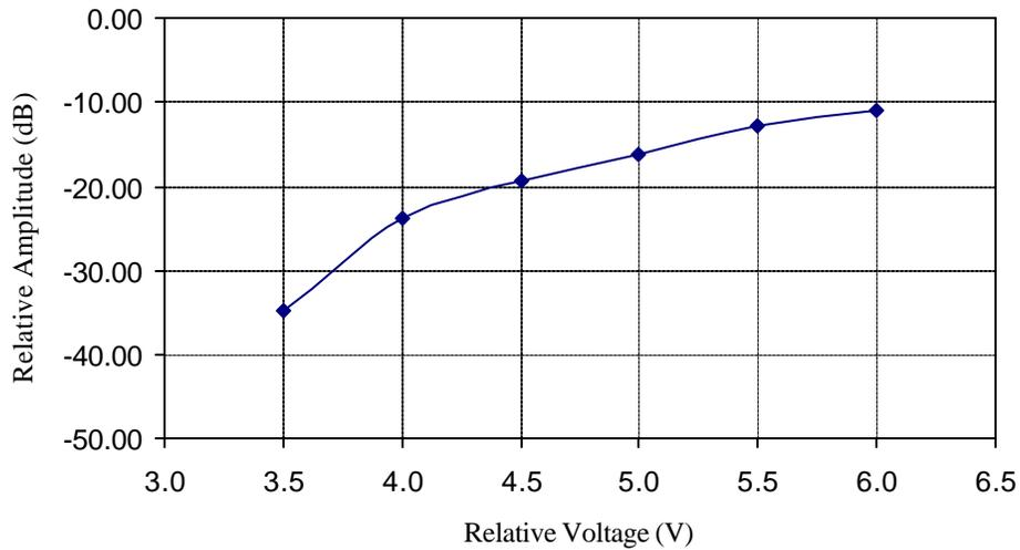
Figure 6.5. Relative emission at 303.0 MHz vs. supply voltage (pulsed emission).
