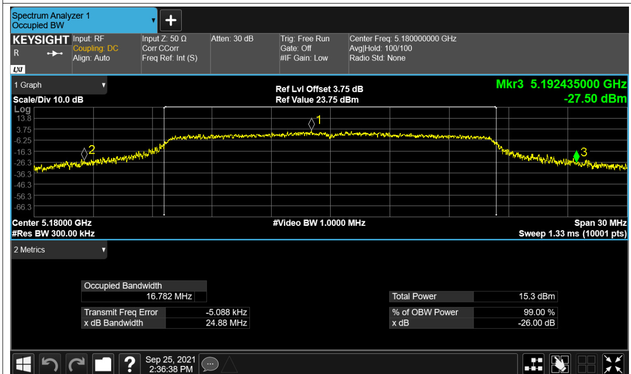
-26dB Bandwidth NVNT a 5200MHz ANT2
