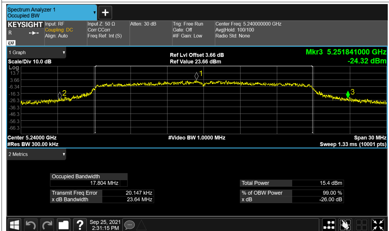
-26dB Bandwidth NVNT ac40 5190MHz ANT1
