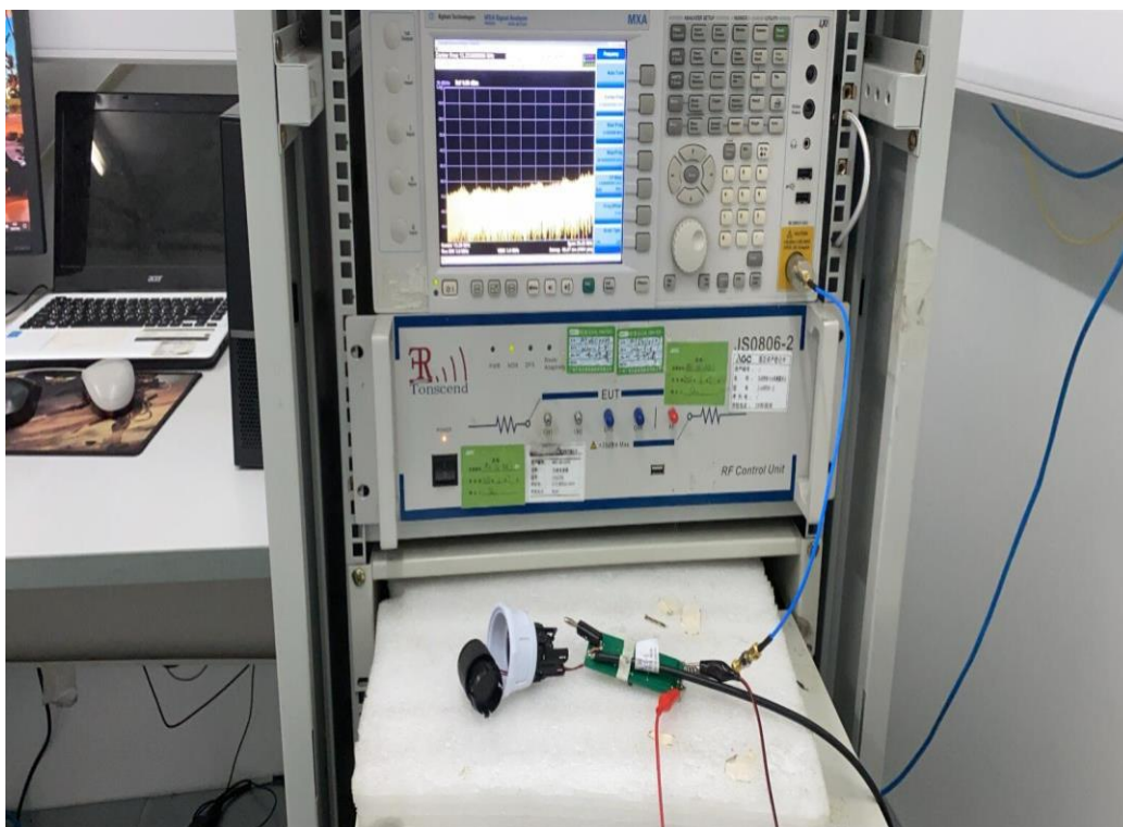
CONDUCTED TEST SETUP-208.5MHz
