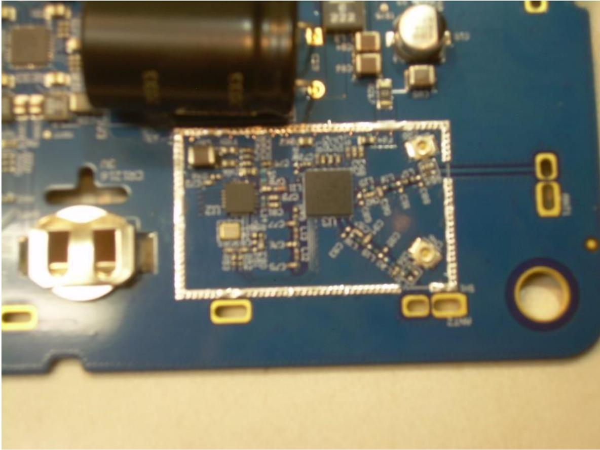
**Photograph 3 – View of Circuitry Under the RF Shield**
