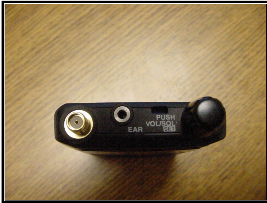
PHOTOGRAPH 13: ANTENNA SMA CONNECTOR
