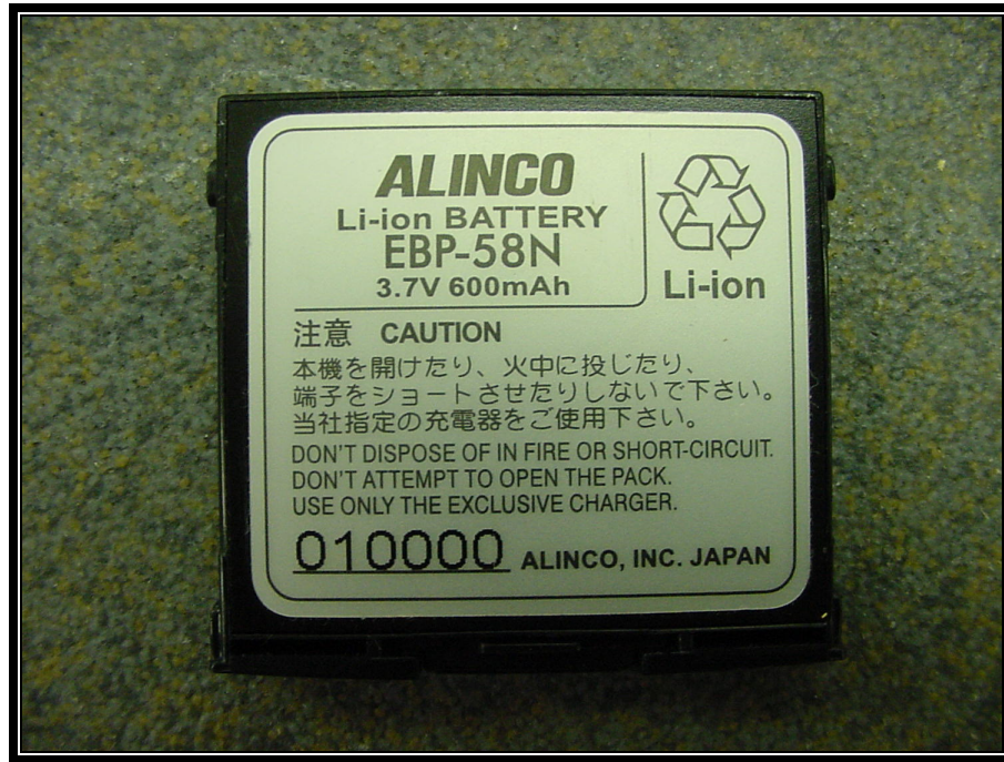
PHOTOGRAPH 11: LABEL ON BATTERY
