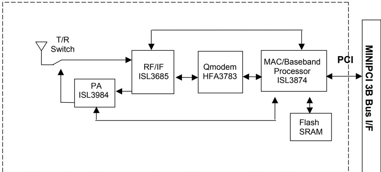
ISL3984:2.4GHz Power Amplifier and Detector
