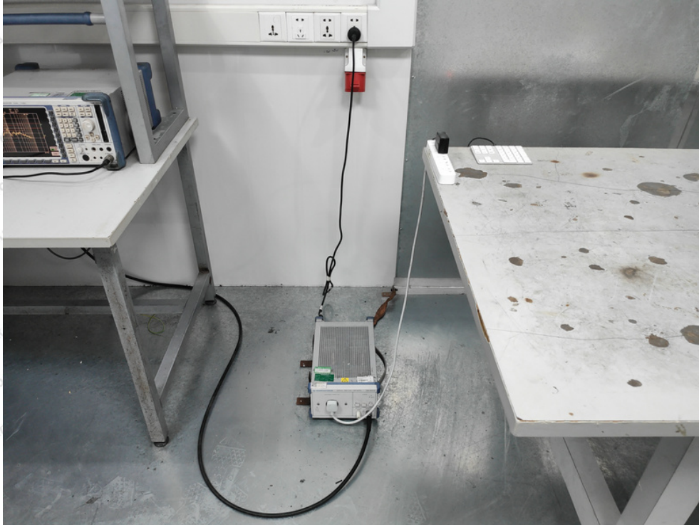
Photo of Conducted Emission Measurement
