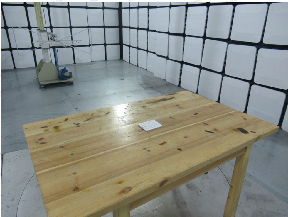
Photo of Radiation Emission Test
