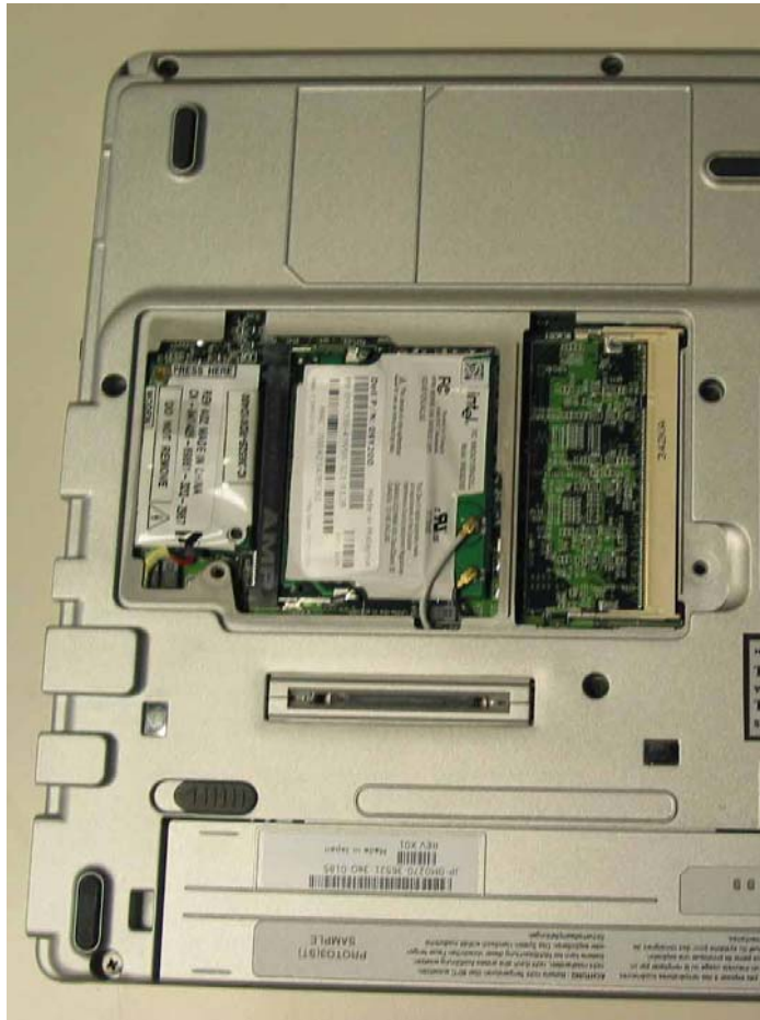
Bottom View showing the MINI PCI expansion slot with (left) and without (right) Wireless LAN Card installed
