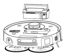
Lift the dust box handle up and take out the dust box.
