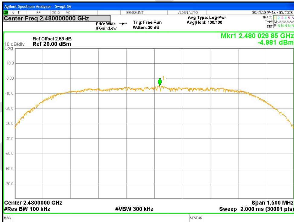
Tx. Spurious NVNT 2-DH1 2480MHz Ant1 Emission
