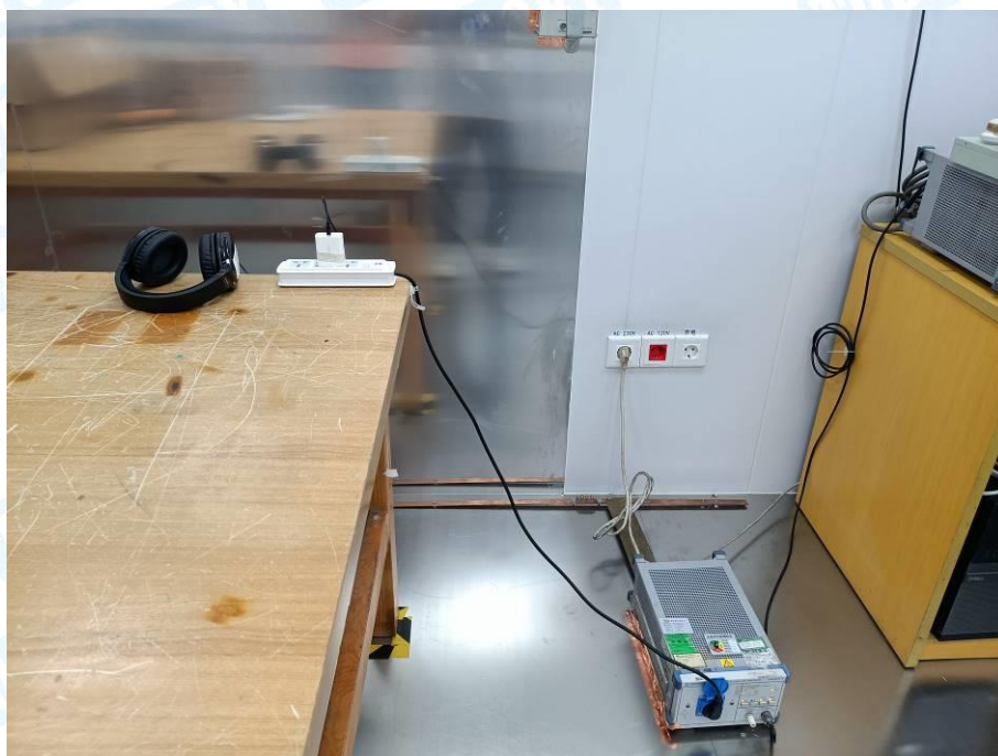
Photo of Setup for Conducted Emission
