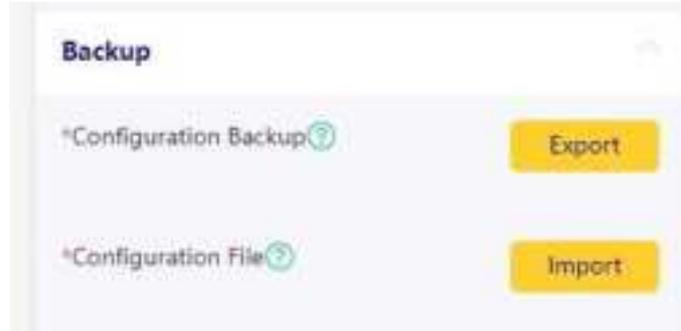
The FST200-00 series supports backing up device configuration information and importing it to other devices for quick batch configuration. The backup information does not include LORA-related parameters and is applicable to batch configuration of products of the same series.
