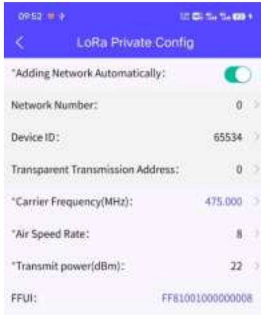
Open the "NFC Configuration --> LoRa Private Configuration" menu in the Sensor Cloud APP, and set the network mode, network number, device ID, pass-through address, carrier frequency, data rate, and transmit power of the device.
