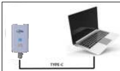
Use type-C to connect the computer to the device. Open the serial port and click Start to Read to obtain the device parameter information.
