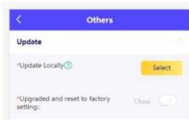
FST200-00 series support NFC upgrade of sensor cloud APP, remote upgrade of Four-Faith sensor cloud platform, and PC configuration tool upgrade. The detailed steps are as follows:
