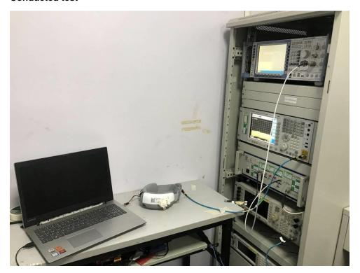
Conducted Emissions at AC Power Line (150kHz-30MHz)
