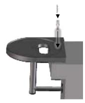
Step 3: Install bracket on sill
