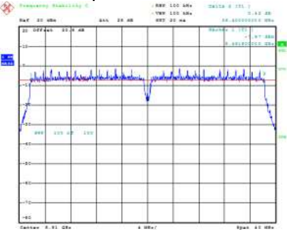
Figure 8-18: 6 dB Bandwidth Secondary, 802.11ac, Channel 100, 6 Mbps
