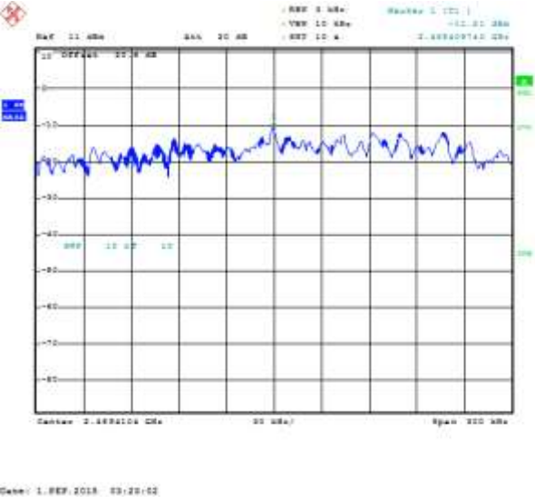
Figure 6-59: Peak Power Spectral Density MIMO Secondary, 802.11n, Channel 6, MCS 0
