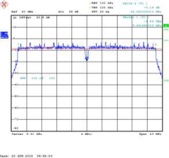
Figure 7-24: 6 dB Bandwidth Primary, 802.11n, Channel 64, MCS 0
