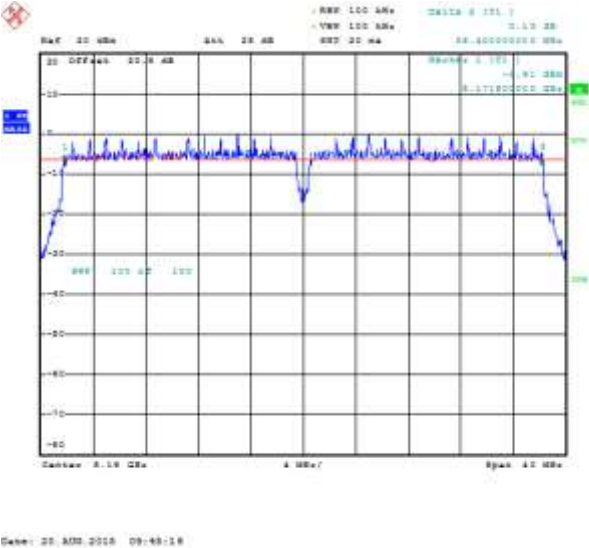
Figure 7-23: 6 dB Bandwidth Primary, 802.11n, Channel 36, MCS 0
