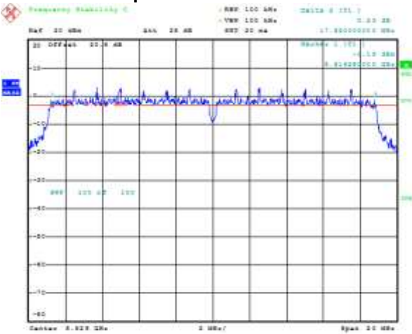
Figure 8-10: 6 dB Bandwidth Secondary, 802.11ac, Channel 149, MCS0 Mbps
