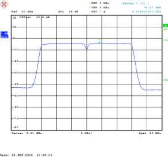
Figure 7-111: Peak Power Spectral Density SISO Secondary, 802.11n, Channel 64, MCS 0
