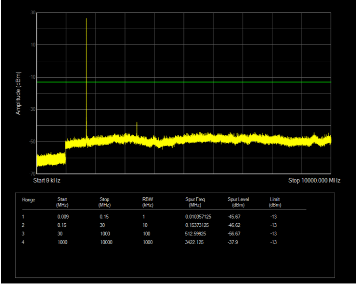
Band66 QPSK BW=1.4MHz Channel=131979 RB Size=6 Position=#0
