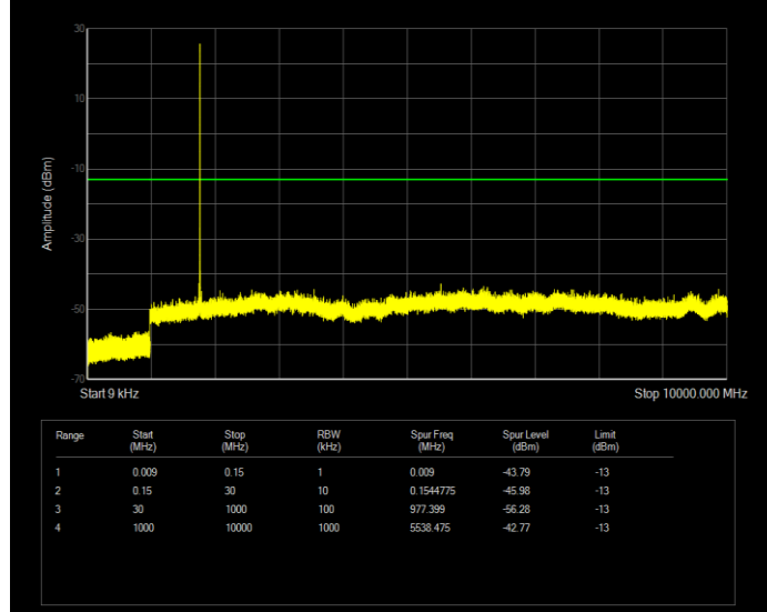
Band66 QPSK BW=10MHz Channel=132022 RB Size=50 Position=#0
