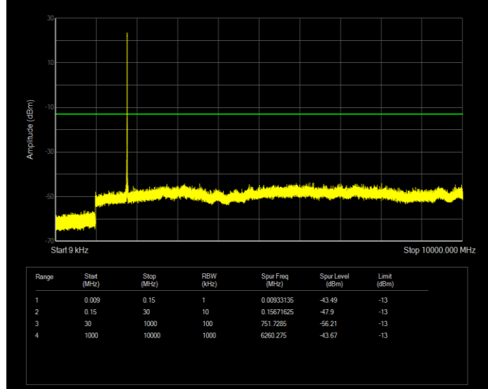
Band66 QAM16 BW=5MHz Channel=131997 RB Size=25 Position=#0
