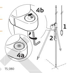
After the adjustments, all adjusting screws must have the same tightening tension and no adjusting screw should be loose.
