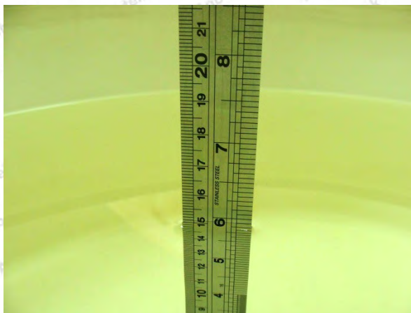
Photo of Liquid Height for Body SAR
