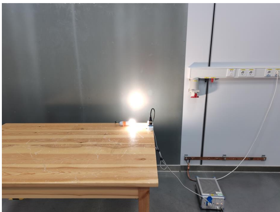
Fig. 4 Power line conducted emission setup photo
