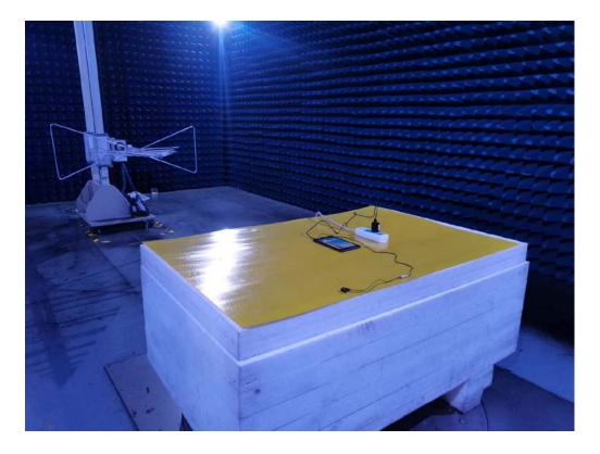
Photo of Radiated Emission Measurement Above 1GHz
